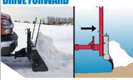
The blade is guided by a push frame that allows it to slide up and down with the grade of the terrain.
