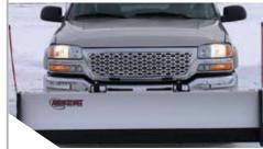
The practical design does not block headlights in plow or transport position.
