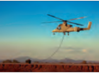
K-MAX features Kaman's high-altitude, heavy-lift K-1200 airframe and Lockheed Martin's mission management and control systems.
