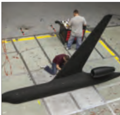
For Phase 2 of NASA's ERA project, Mehdi Khorrami's team is testing flap and landing gear noise-reduction technologies using a half-span, 18%-scale model of a Gulfstream G550 installed in Langley's 22x14-ft wind tunnel.
