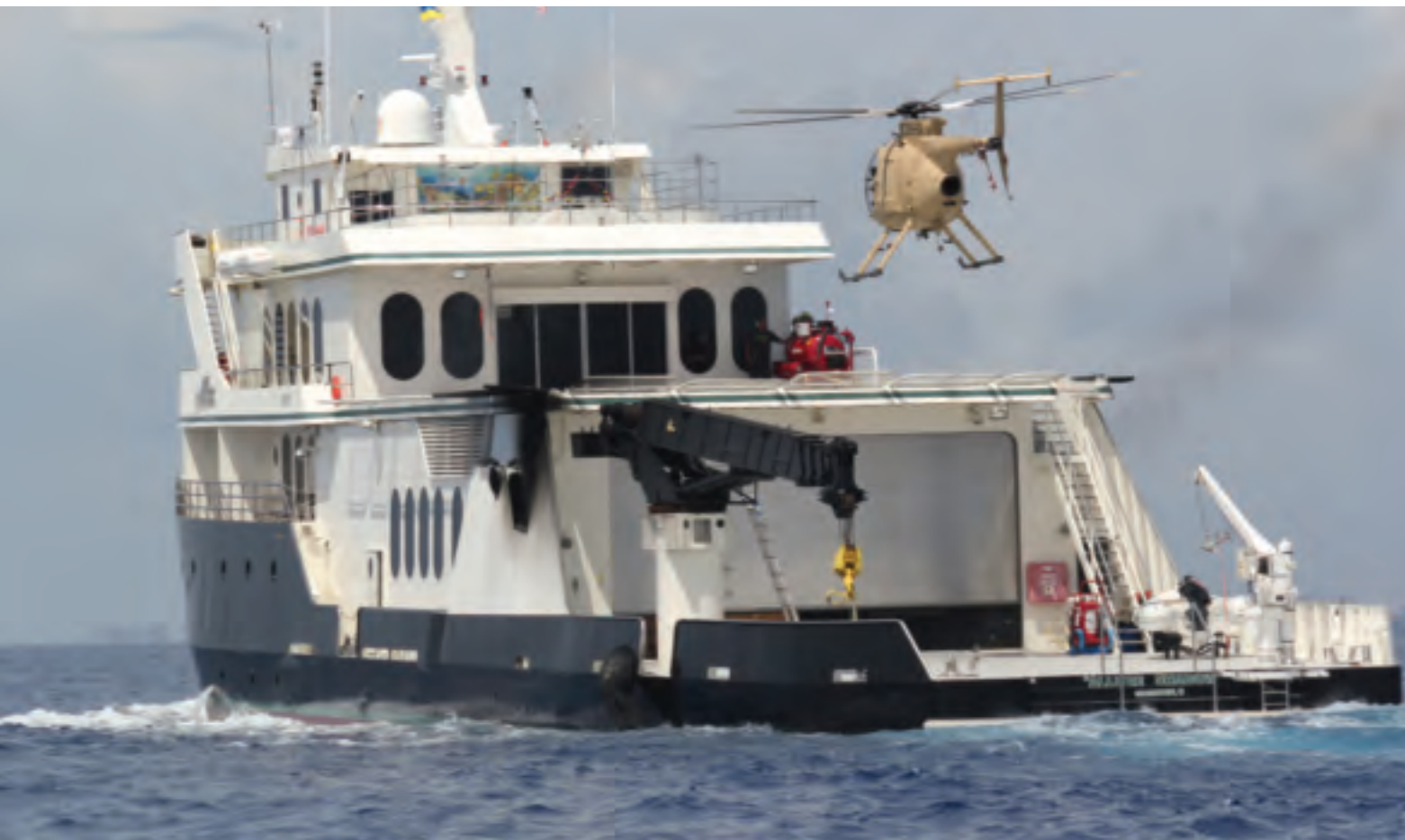
Unmanned Little Bird successfully performed 14 autonomous takeoffs and landings from a ship during flight tests in July 2012.
