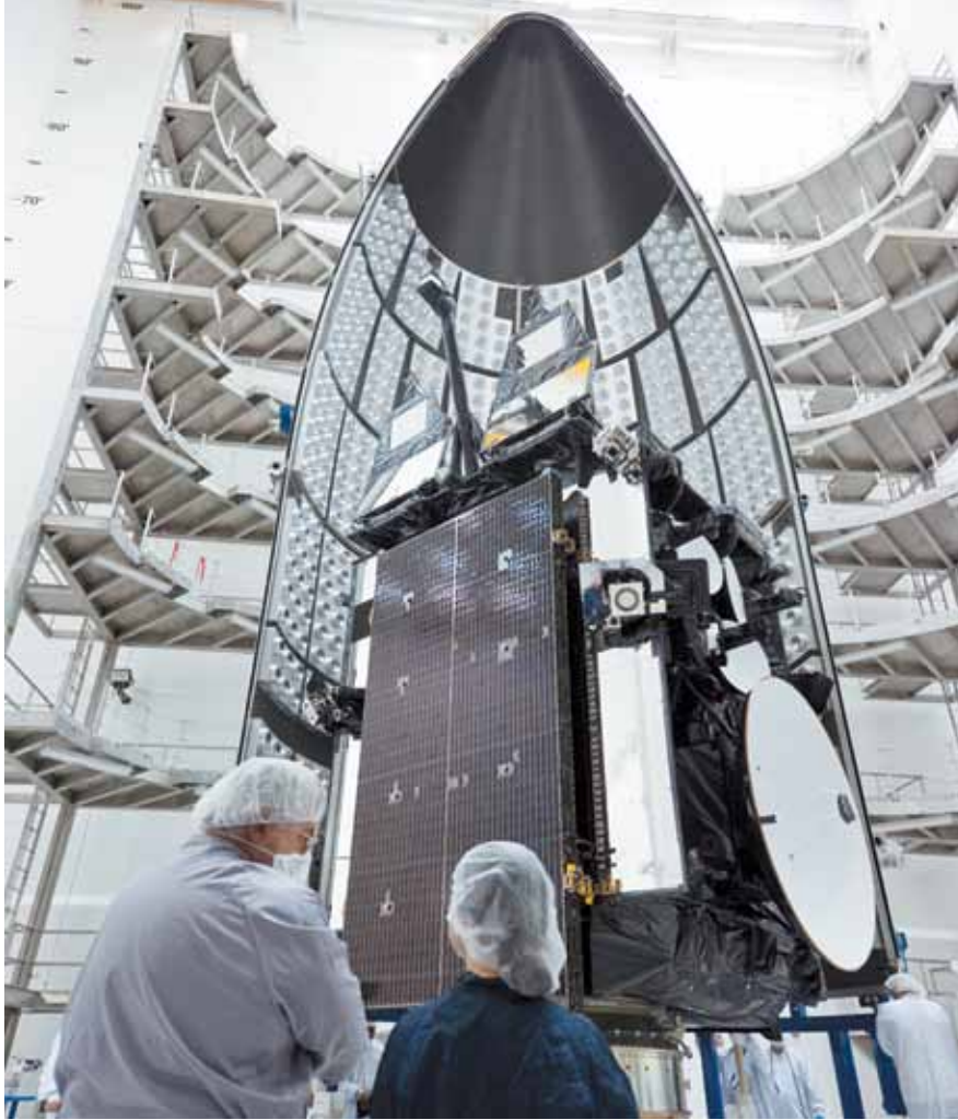
A look inside the Atlas V payload fairing while the second Advanced Extremely High Frequency satellite is encapsulated. Shelton is pleased by the progress of the new generation of satellites such as AEHF, but feels more attention must be paid to the survival of the actual platform.
