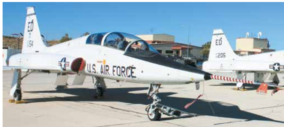
A pair of T-38s on the flight line have fully instrumented nose probes that allow TPS students to collect data during test training hops.
