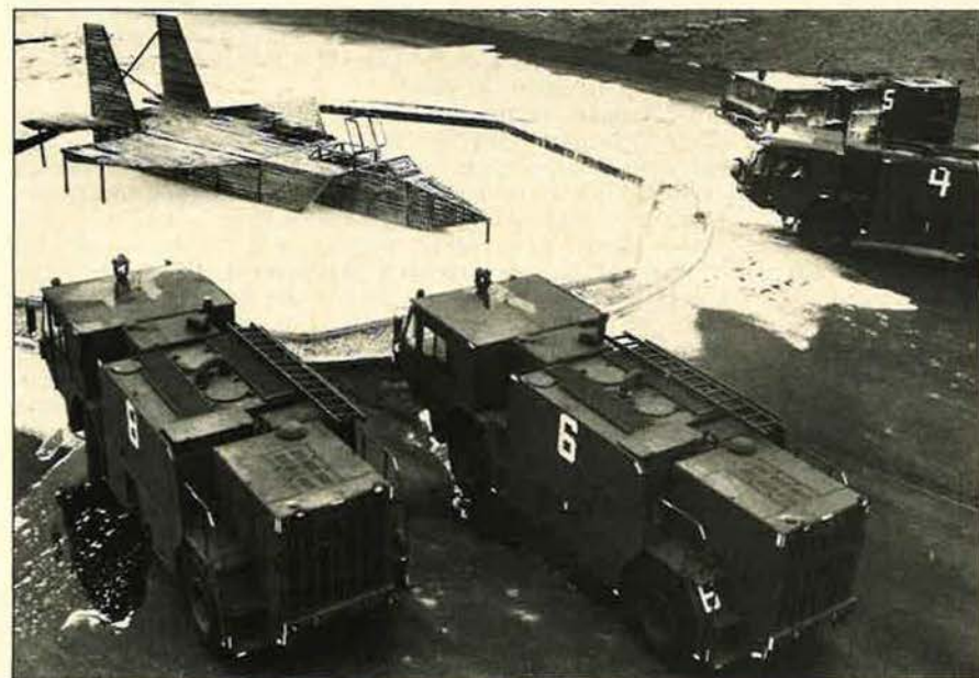
This "F-15" will live to see another "crash." Four P-19 fire trucks from the Bitburg AB, West Germany, Fire Department put out a fire in the base's prototype training pit, a thirty-foot-diameter concrete circle with paved approaches.
