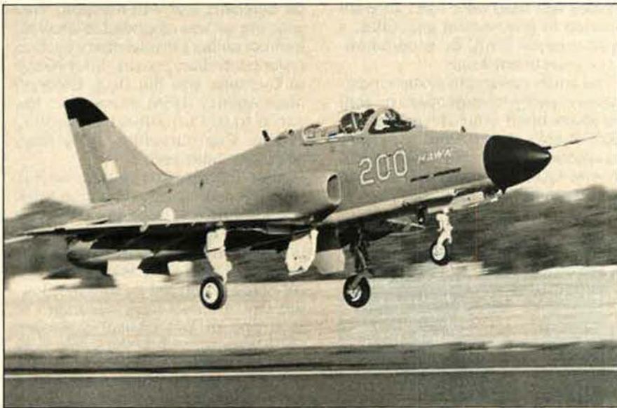
British Aerospace's new single-seat lightweight fighter version of the Hawk trainer, the Hawk 200, made its first test flight on May 19. Test pilot Jim Hawkins was killed in the crash of the prototype on July 2. Another Hawk 200 will be built.
