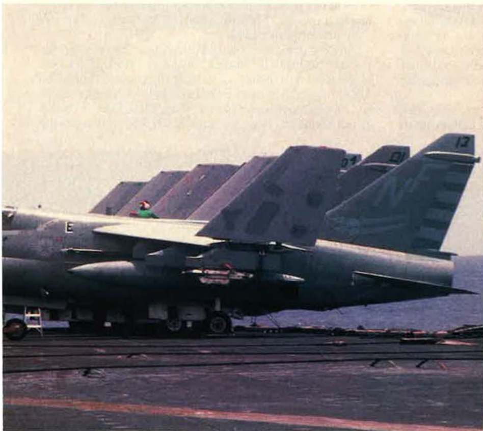
Navy A-7 Corsair II aircraft played a significant role in recent events in the Gulf of Sidra. The venerable A-7s were first used in Vietnam and have grown in lethality with the use of AGM-88A High-speed Anti-Radiation Missiles (HARMs). Now nearing the end of their shipboard service life, the A-7s will eventually be replaced with F/A-18s. These aircraft are assigned to the USS Midway (CV-41) in the Pacific.
