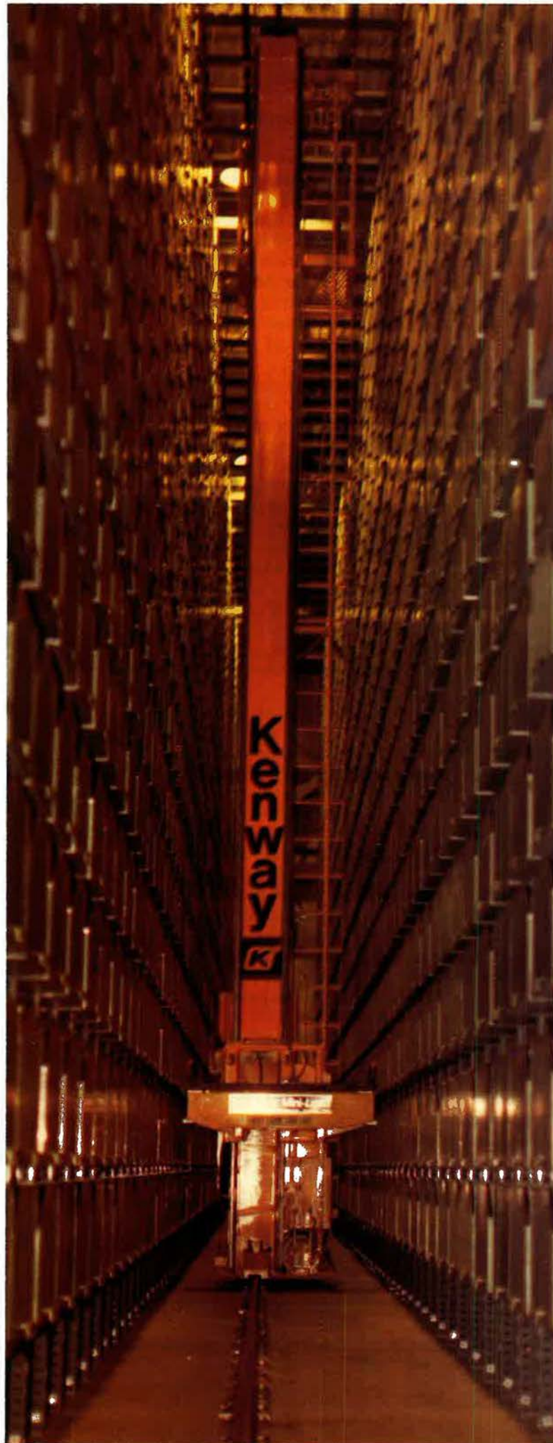
A view of automated storage modules at the Ogden Air Logistics Center, Hill AFB, Utah. One LMS project, the Stock Control & Distribution System, will tie together such already completed warehouse upgrades and significantly cut down depot processing time. (USAF photo)
