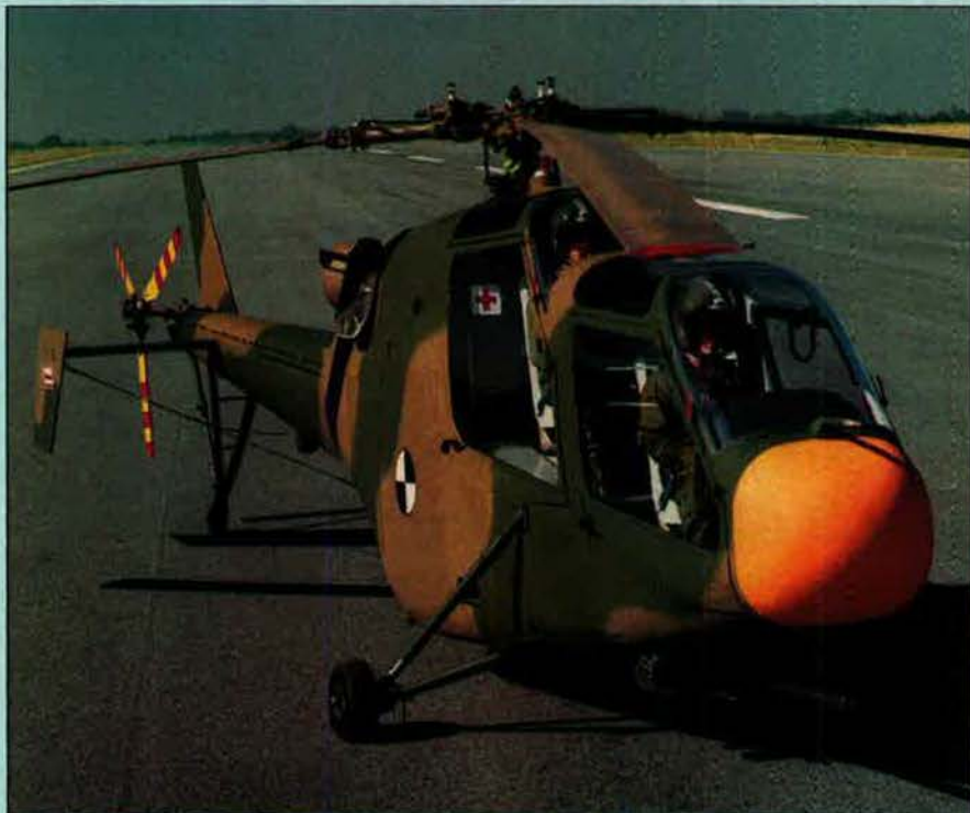
The good all-round field of view for the two-man crew is evident in this photograph of the Atlas Alpha XH-1
