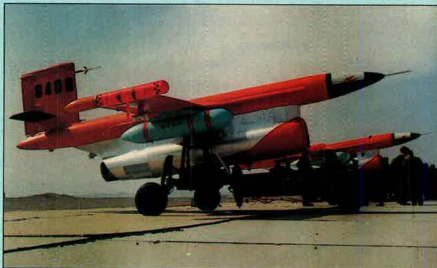
NAI Changkong 1C (CK1C) highly manoeuvrable and recoverable target drone ( Wang Lue )
