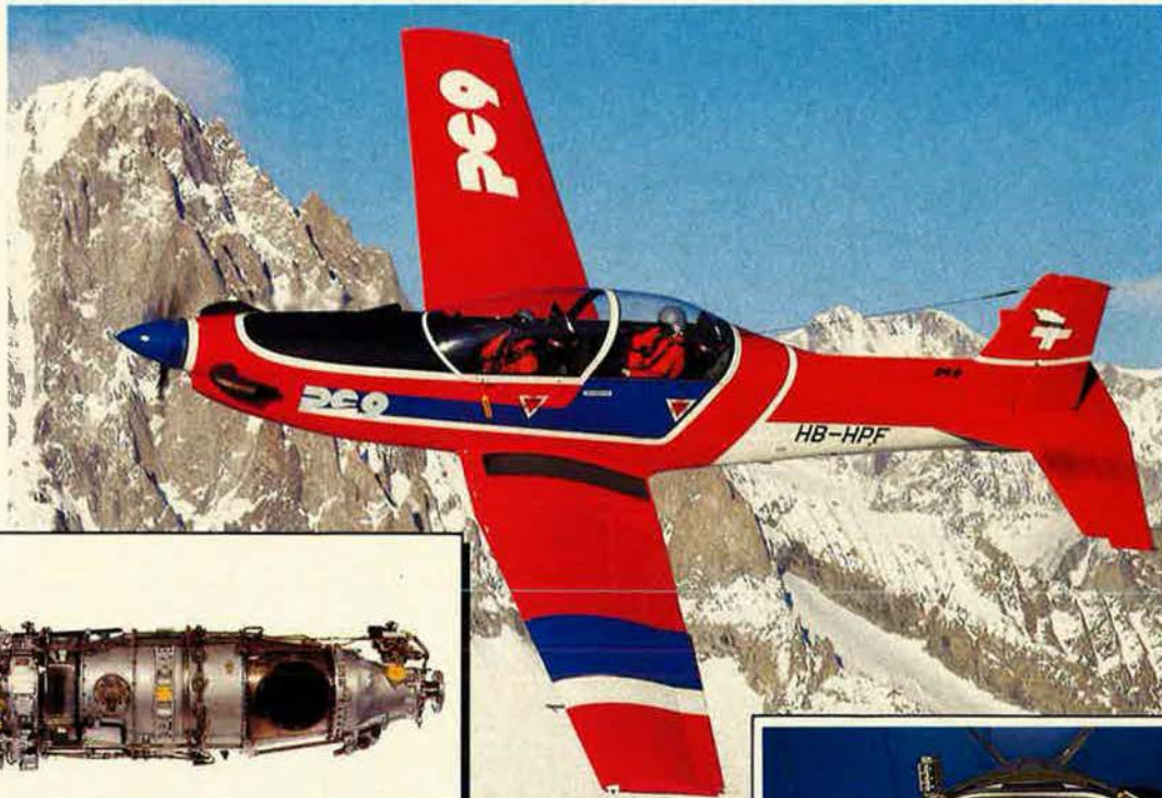
Latest technology 1,150 shp, derated to 950 shp, Pratt & Whitney PT6A-62 engine is fitted with electronic temperature and torque limiter.
