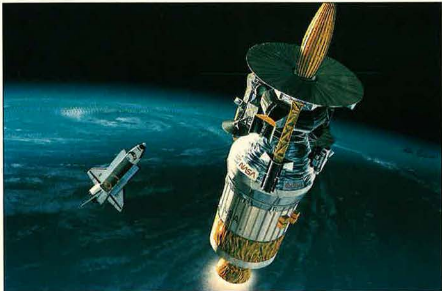
This artist's concept shows the Galileo Jupiter probe atop its Air Force-developed Inertial Upper Stage after it was released from the space shuttle Atlantis on the recent STS-34 mission. Air Force crews aboard the 4950th Test Wing's EC-135N aircraft provided telemetry data during the launch.
