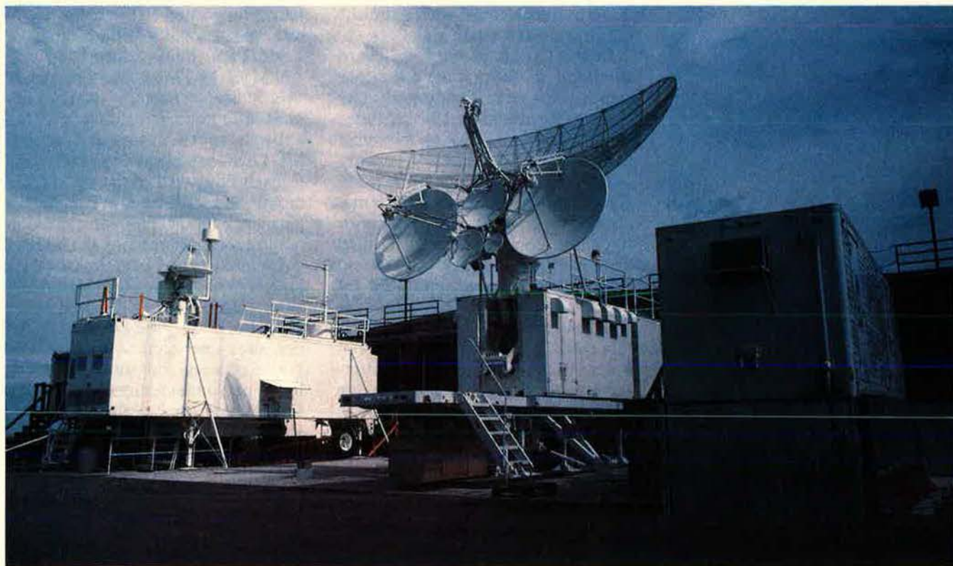
Six permanent radar bomb scoring sites, such as this one near Belle Fourche, S. D., are scattered over the fourteen low-level training routes that make up the Strategic Training Route Complex. Shown are the MUTES and TRAINS, a pair of systems that first imitate the signals of up to ninety threat radars and then record the bomber crew's reaction to those signals.
