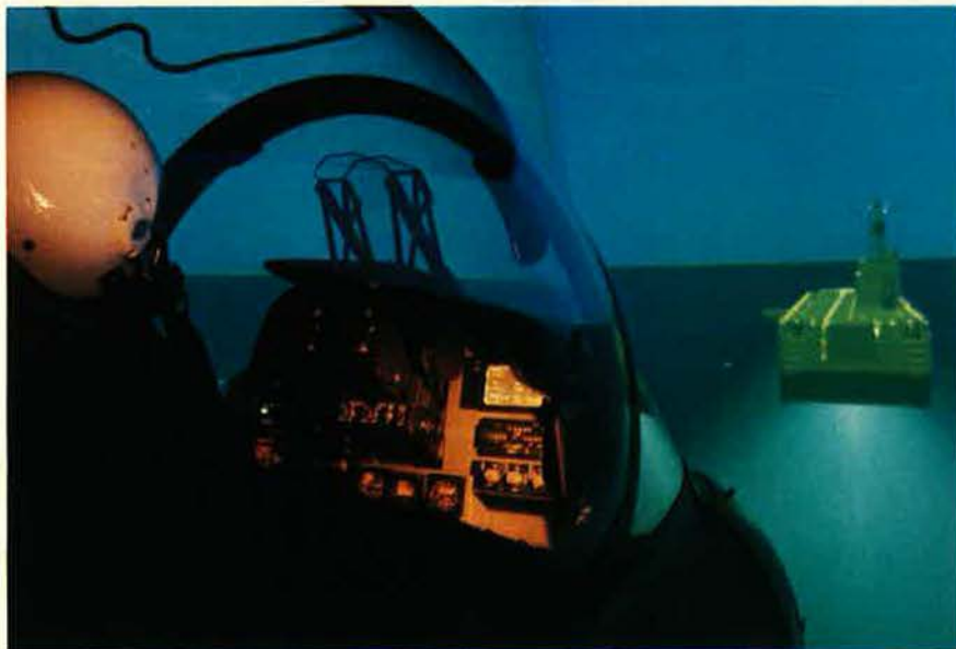
At the Marine Corps Air Station, Cherry Point, N. C., a Marine Corps pilot in a McDonnell Douglas Operational Flight Trainer lands an AV-8B Harrier II light attack aircraft on a deck of a simulated carrier. The trainer's digital recording system adds realistic sound as part of the mission simulation.
