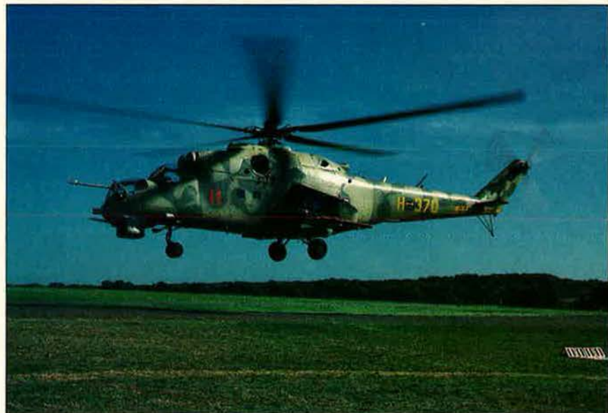
The latest version of the Soviet Hind attack helicopter made its Western debut at the Helltech Exposition in Redhill, England, in September. This example, billed as an export "MI-35P," features a twin-barrel 30-mm cannon on the starboard side of the nose, four underwing pods carrying twenty 80-mm rockets each, and four AT-6 Spiral antitank missiles. The twin-engine helicopter was shown without its infrared protection equipment, which includes a jammer and exhaust deflectors.
