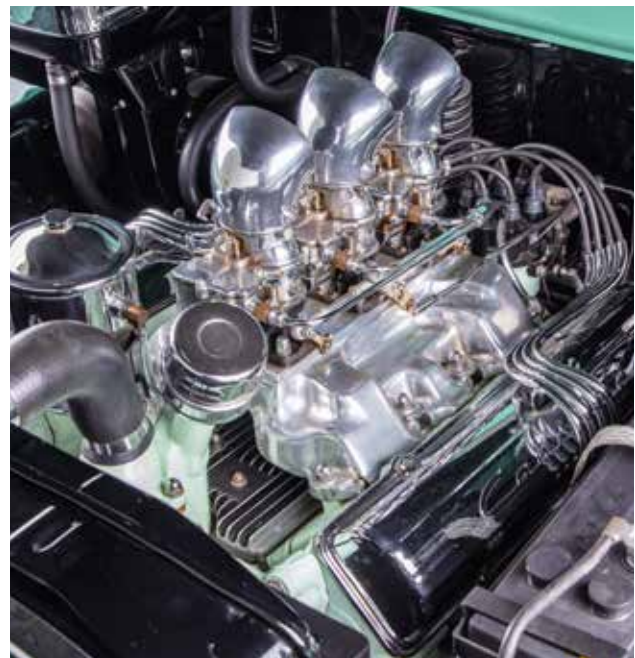
The Hirohata's interior and trunk were done by two trimmers: Glen Houser's Carson Top Shop and Bill Gaylord. Its Cadillac V-8 has a three-carb intake manifold and an Iskenderian cam.
