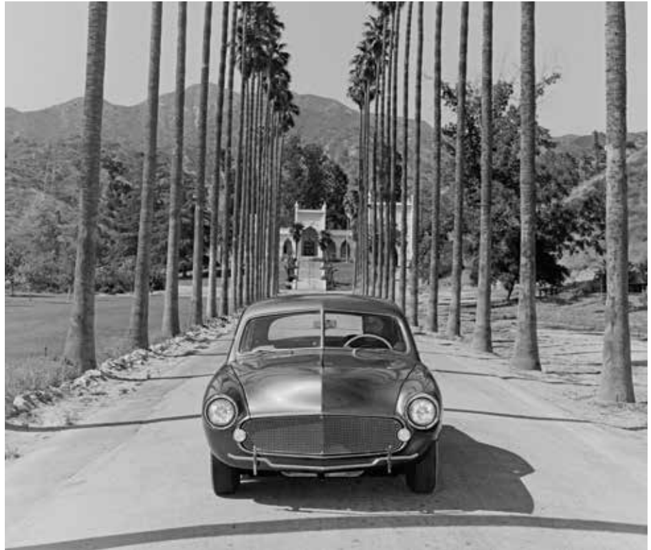
Left: “The Polynesian,” a sectioned 1950 Oldsmobile Holiday 88. Above: Valley Custom sectioned this 1951 Ford in 1953. In its second iteration, chrome nerf bars replaced the stock bumpers.
