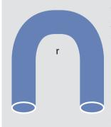
The bend radius is the radius of the arc through which a hose is bent. The minimum bend radius is the tightest arc in which a hose can be bent without kinking or otherwise damaging the hose.
