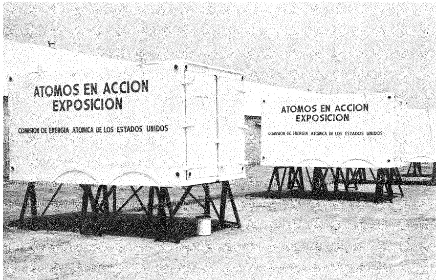
Truck van bodies converted to sea lifts for shipping AEC exhibits of Atoms-at-Work to Central and South America.
