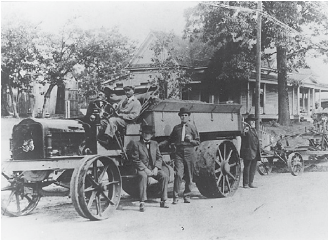
One of the first pull road graders in Camden in the 1920's.
