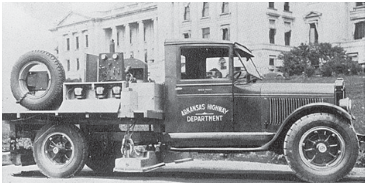
Metal objects which could puncture tires were collected from the roadways by magnet trucks. A sign on the back indicated that these trucks picked up an average of 20 pounds of metal per mile.
