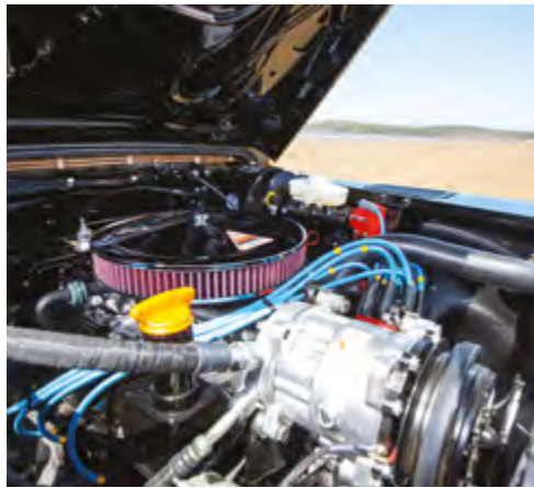
3.5L V8 fully reconditioned engine with additional fuel injection
