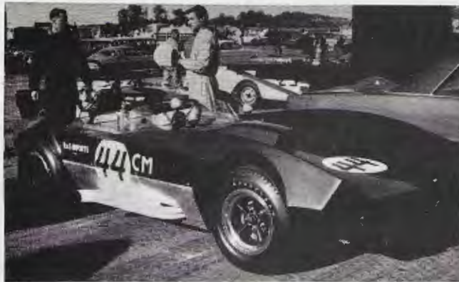
Above: Al Schall (left) and Carliss (right) will share driving chores in coming season's racing. As seen here the car was fitted with Carter carb. setup, complete with neat air scoop in front of the windshield.
