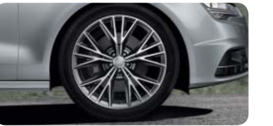
Forged aluminium wheels in 5-spoke W design, contrasting grey, partly polished 2 size 9 J x 20 with 265/35 R 20 tyres 1
