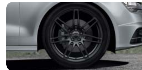
Audi Sport forged aluminium wheels in 7-twin-spoke design in gloss anthracite black 2,3 size 9 J x 20 with 265/35 R 20 tyres 1
