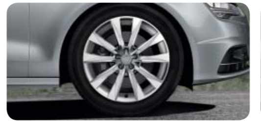
Cast aluminium wheels in 5-spoke V design size 8.5 J x 19 with 255/40 R 19 tyres 1 , optionally available with run-flat tyres
