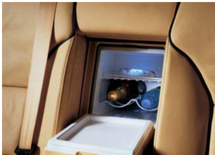
Personal Refrigerator in pass through
