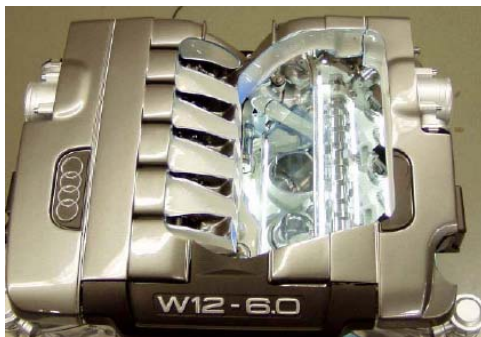
Intake manifold - new design, optimized length
