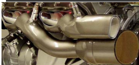
One unit: air gap insulated exhaust manifold and 3-way catalyst in close proximity to engine
