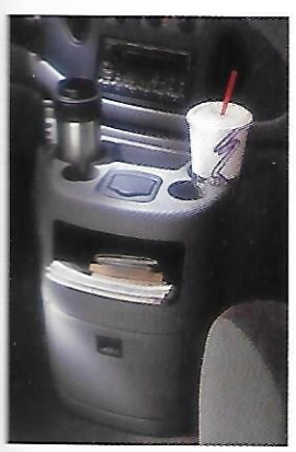
The restyled deluxe engine cover console includes two storage areas, four cupholders, a juice box holder/ashtray, coin slots, and a bin designed to accommodate a cellular phone.
