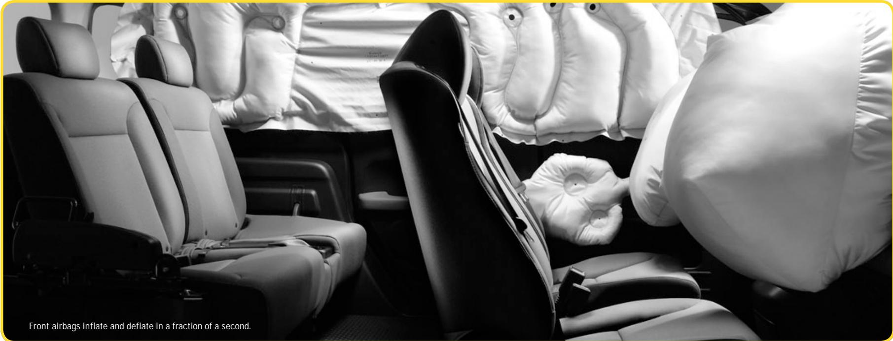
Front airbags inflate and deflate in a fraction of a second.
