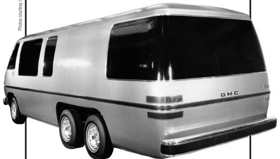
During the GMC Motorhome design phase, clay models were created to test different ideas, among them the 1/8-scale model above, shown with a full-size tape drawing and various sketches in the background. These led to the production of a full-size clay model, known as RV-26 (pictured top and bottom); note the wraparound taillights and rear window styling of this model.
