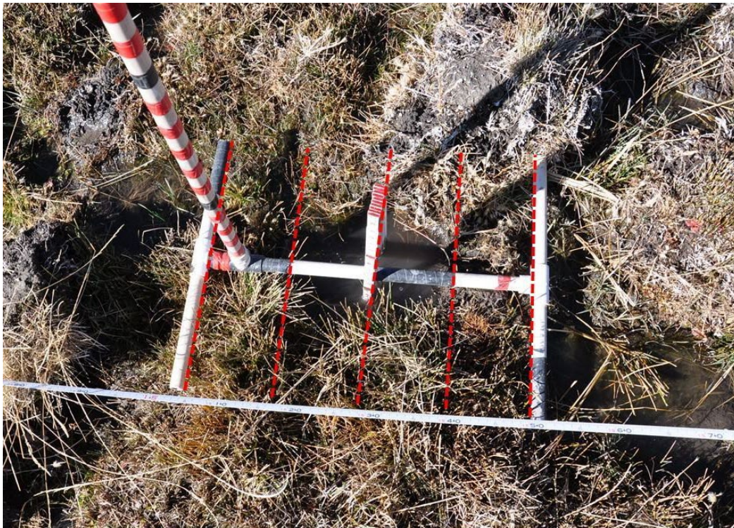
Figure 51. Soil alteration is evaluated by projecting five lines (red dashed lines) across the frame and perpendicular to the center bar. Two lines coincide with the outer cross pieces of the frame, and three inner lines are spaced 12.5 cm apart. In this example, soil alteration would be recorded as 3 because the second, third, and fifth lines intersect soil alteration. The second and third lines both intersect the same large hoof print.
