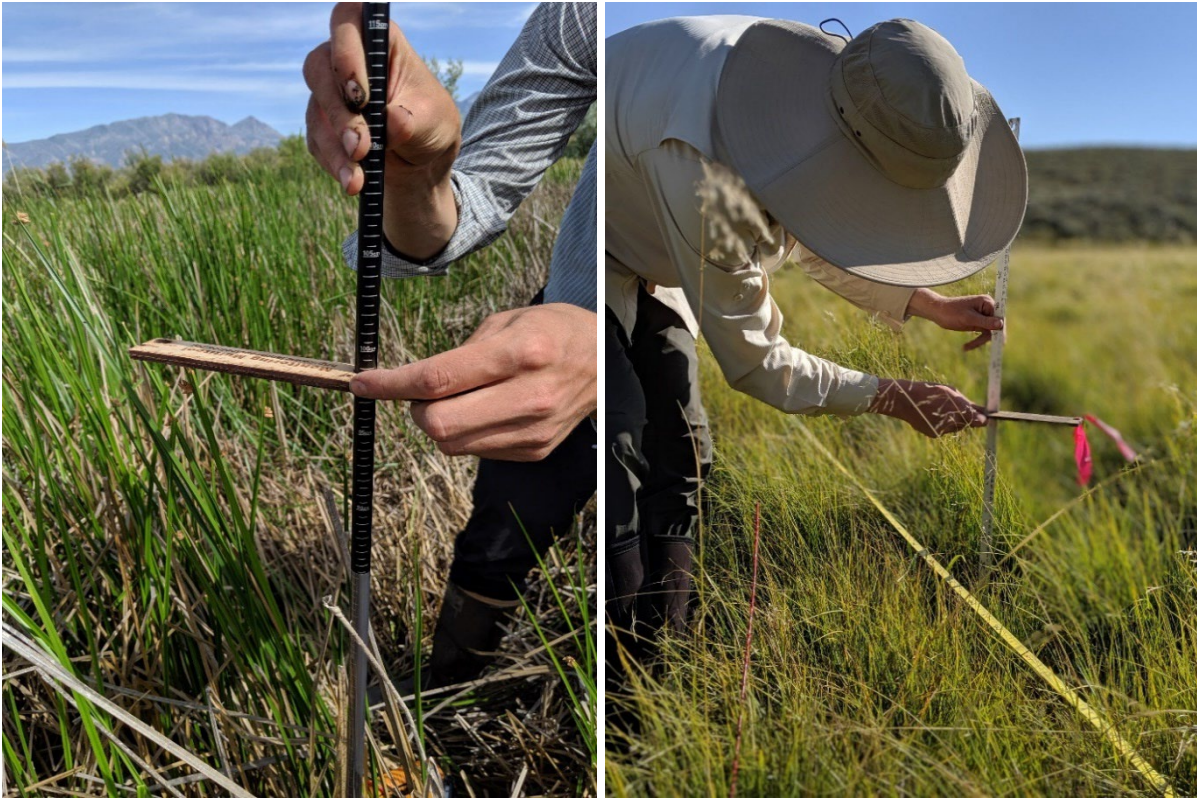
Figure 34. Measuring vegetation height and litter and water depths using a measuring rod and a ruler notched to create a 15-cm radius circle.
