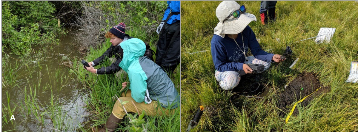
Figure 47. Measuring pH, specific conductance, and temperature with a water quality probe in (A) surface water and (B) groundwater within a soil pit.
