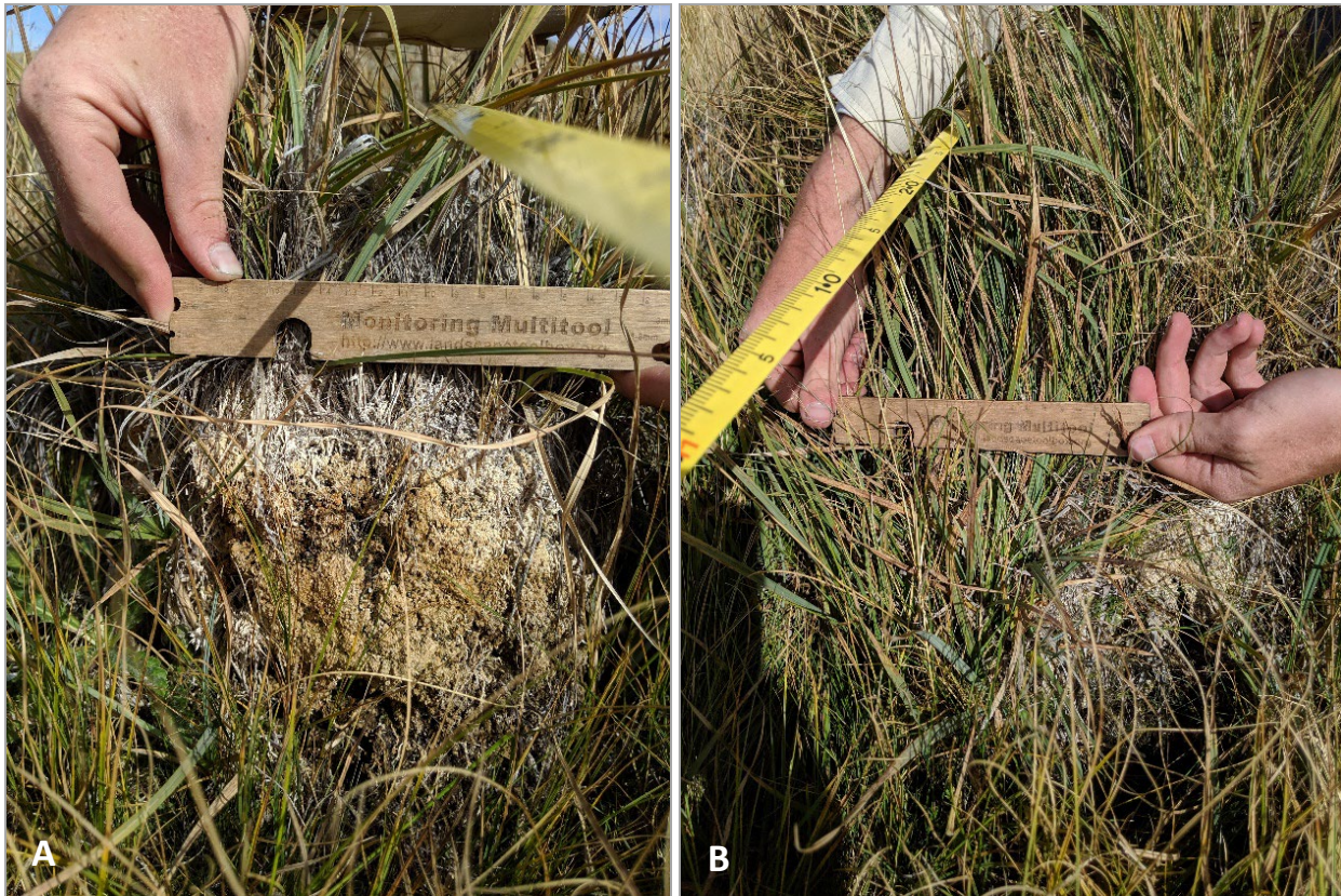
Figure 43. Estimating vegetation canopy cover on the leading edge of a hummock. Delineate a box from the base of the hummock to the shoulder and extending 10 cm on either side of the tape. Photos show (A) an unvegetated slope and (B) a mostly vegetated slope.
