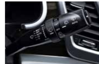
Multi-function control switches
