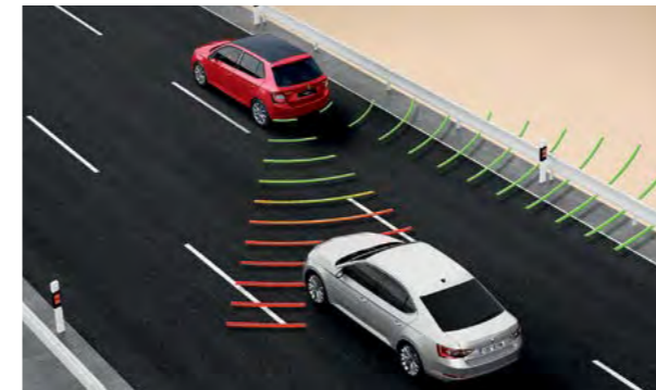
BLIND SPOT DETECTION WITH REAR TRAFFIC ALERT
