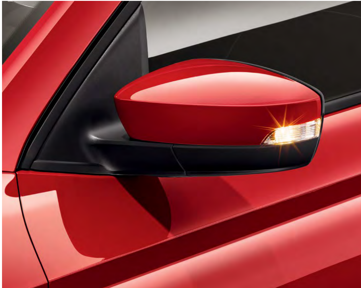
ELECTRICALLY ADJUSTABLE AND HEATED DOOR MIRRORS
