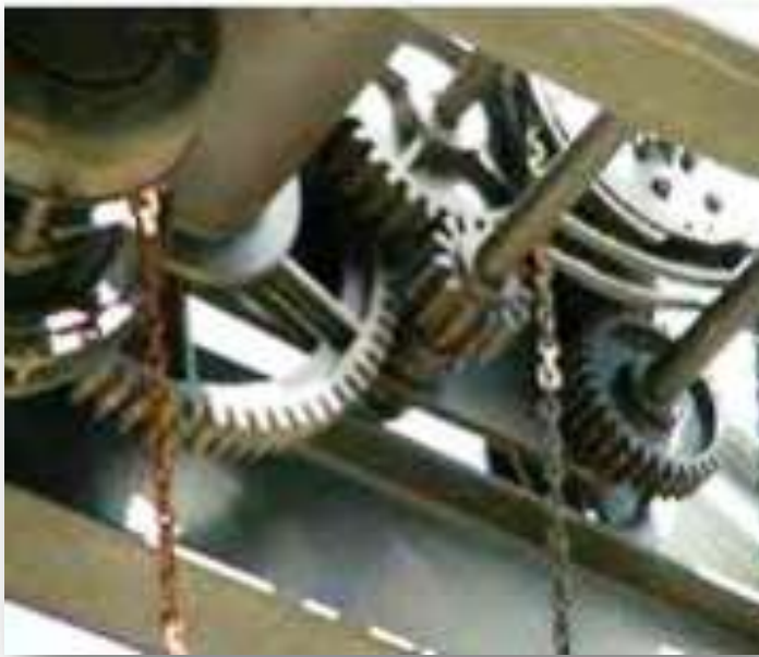
19. Gantry Hoist now incorporated into Jacksons Landing Development, Pyrmont. It is a reconstruction of a workshop portal frame, supporting a gantry hoist from the Engineers workshop. Source: Site Interpretation Strategy: Jacksons Landing, Pyrmont August 2003.
