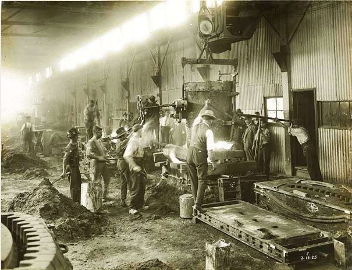
53. Pouring first steel casting at Hadfield's Works 1925. The man in a suit on right is thought to be JJ Bradfield. Source: State Records Series No 12685
