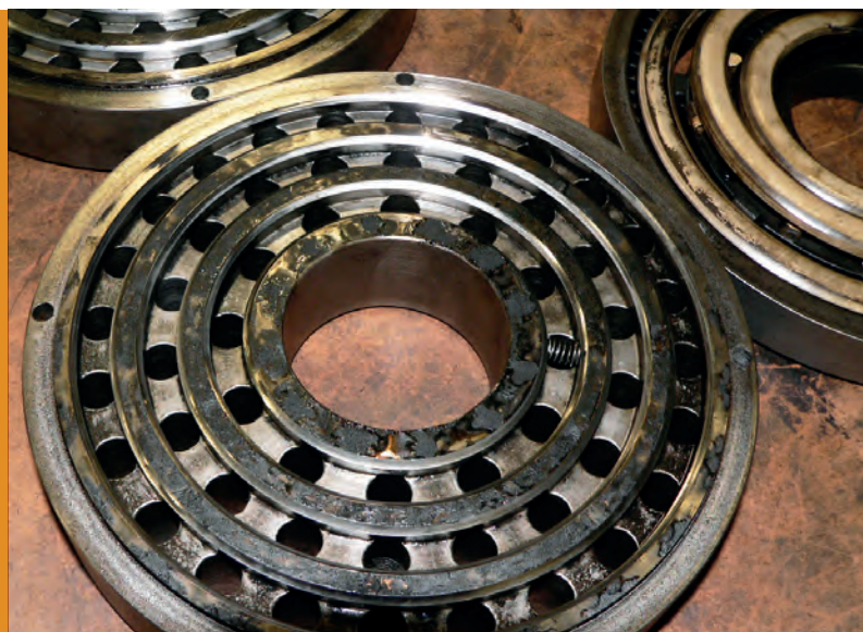
FIGURE 13 Oil residue (sometimes in a burnt-on carbon form) is often evidence of excessive lubrication oil in a compressor valve.
