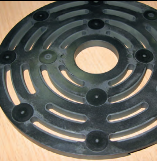
FIGURE 2 A mottled witness pattern on the back face of a valve plate might indicate excessive opening impacts.
