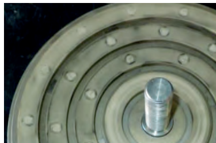
FIGURE 4 Spring fatigue failure may result from excessive valve flutter cycles.
