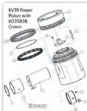
The KVTR two-piece piston assembly.
