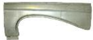
Wheel Arch Repair
