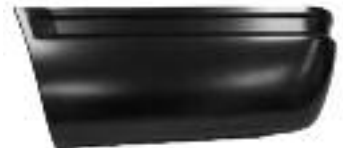
Rear Section Behind Wheel, Suburban
