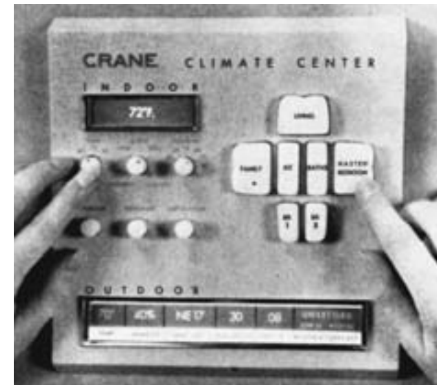
Above: You could take your pick of fragrance—seashore or northern woods—and any temperature or level of humidity you wished, on the “House of the Future” Crane Climate Center panel. Even outdoor temperature and forecasts could be quickly determined.
