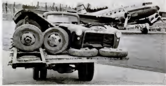
PIECES OF TRUCKS which have been disassembled and cut up with torches so that they will fit in planes are brought to an Ungava DC-3 for the trip to Knob Lake. When they get to Knob Lake they will be welded together and reassembled.
