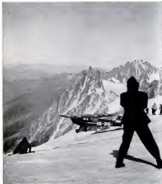
SUCCESSFUL TAKE-OFF was made 10 days later after repairs were done. Guides stretched a rubber rope (lying under plane) to catapult it into the air.
