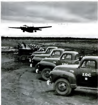
BIGGEST TIMESAVER is this C-119 Flying Boxcar which the company borrowed from U. S. Air Force to speed up shipments. When this plane is used trucks and Harvester tractors in foreground can be flown in without being disassembled.
