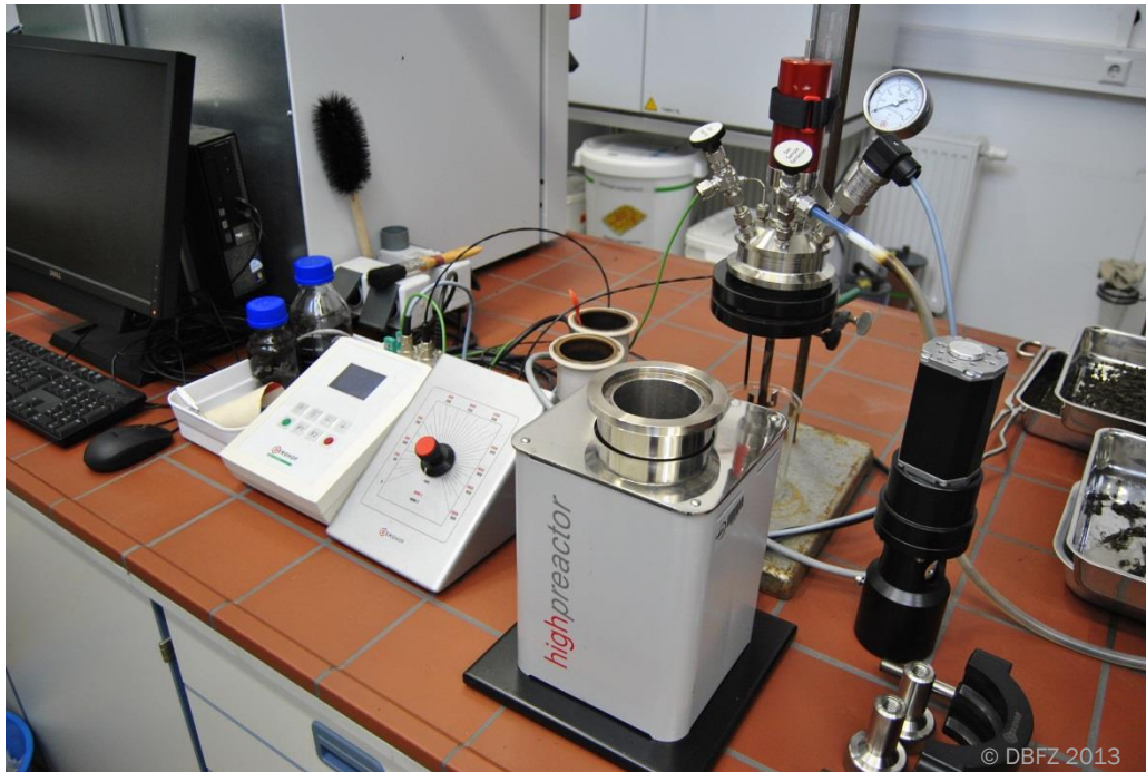
Figure 6.1 HTC test stand
