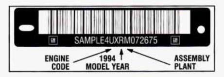
This is the legal identifier for your Buick. It appears on a plate in the front corner of the instrument panel, on the driver's side. You can see it if you look through the windshield from outside your vehicle. The VIN also appears on the Vehicle Certification and Service Parts labels and the certificates of title and registration.
