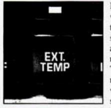
Push this and the display will indicate the outside temperature (unless the system is OFF). Push it again to return to the regular system display. The outside temperature reading is most accurate when driving. During stops, the display shows
