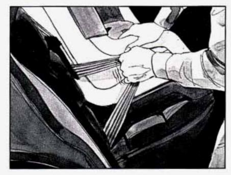
To tighten the belt, feed the lap belt into the retractor while you push down on the child restraint.
