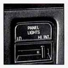
The instrument panel intensity can be adjusted by moving this lever between "LO" and "HI". The interior courtesy lights can be turned on by sliding the lever all the way to the right.
