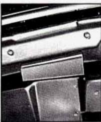
The hood latch is located under the hood, near the center, and at the front edge of the grille.
