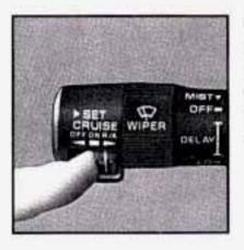
Once you're going about 25 mph (40 km/h) or more, you can move the Cruise Control switch from "ON" to "Resume/Accelerate" for about half a second.
