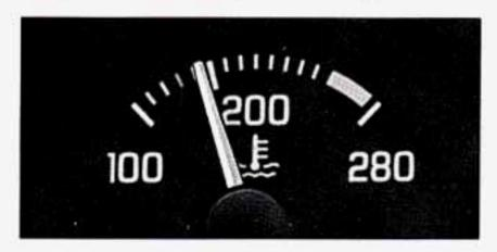
If you have the gage cluster, you have a gage that shows the engine coolant temperature. If the gage pointer moves into the red area your engine is too hot!
