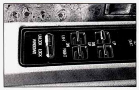
Your power window controls are on the armrest. The switch for the driver's window has an express-down feature. Hold the switch down all the way, release it and the window will lower automatically. To stop the window, from lowering push the switch again. To partially open the window, push the switch and quickly release it.
