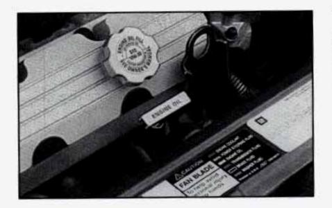
The engine oil dipstick is directly behind the engine fan.
