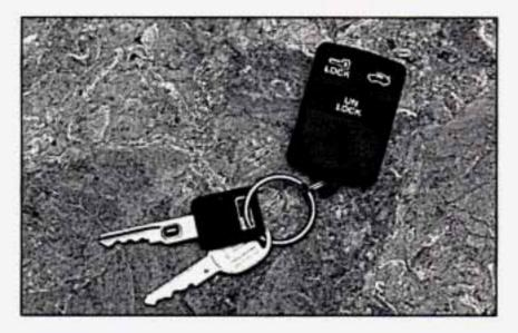
If your Buick has this option, you can lock and unlock your doors or unlock your trunk from up to 30 feet (9 m) away using the key chain transmitter supplied with your vehicle. Your Remote Keyless Entry System operates on a radio frequency subject to Federal Communications Commission (FCC) Rules.
