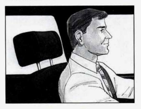
Slide the head restraint up or down so that the top of the restraint is closest to the top of your ears. This position reduces the chance of a neck injury in a crash.
