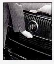
Then go to the front of the vehicle and release the secondary hood latch.
