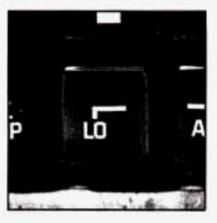
If you want the blower fan to run at a lower speed, push the LO button. The fan speed will decrease with every push of the button until the lowest speed is reached.
