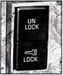
Push the power door lock switch to lock or unlock all the doors at once.
