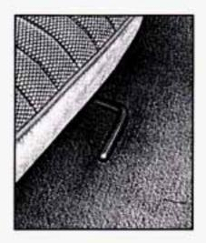
Move the lever under the front seat to unlock it. Slide the seat to where you want it. Then release the lever and try to move the seat with your body, to make sure the seat is locked into place.
