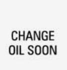
This light is activated by the Engine Oil Life Monitor System. The Engine Oil Life Monitor determines the condition of the engine oil and lets you know when the oil should be changed. See "Engine Oil" in the Index.
