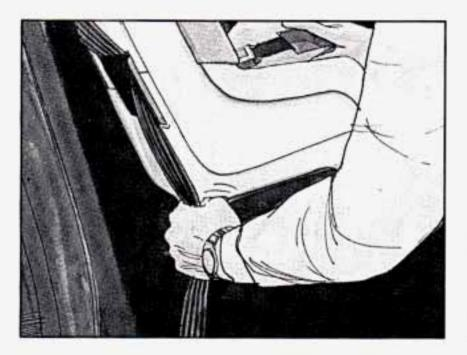
To tighten the belt, feed the lap belt back into the retractor while you push down on the child restraint.
