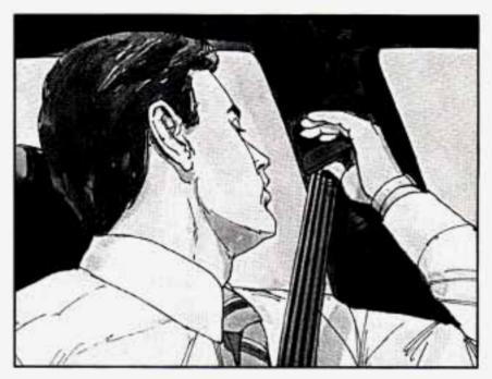
To move it up or down, squeeze the release handle. When you release the handle, try to move it down a little to make sure it has locked into position.
