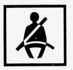
When the key is turned to "Run" or "Start," a chime will come on for about eight seconds to remind people to fasten their safety belts. The safety belt light will also come on and stay on for about 70 seconds. If the driver's belt is already buckled, neither the chime nor the light will come on.
