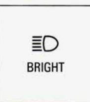
To change the headlights from low beam to high or high to low, pull the turn signal lever all the way toward you. Then release it. When the high beams are on, this blue light on the instrument panel also will be on.
