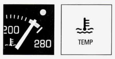
This light tells you that your engine coolant has overheated or your radiator cooling fans are not working. If you have been operating your vehicle under normal driving conditions, you should pull off the road, stop your vehicle and turn the engine off as soon as possible.
