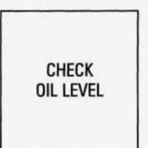
If the "CHECK OIL LEVEL" light on the instrument panel comes on, it means you need to check your engine oil level right away.
