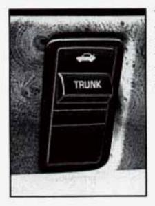
The "TRUNK" button is on the instrument panel to the left of the steering column. The transaxle must be in PARK or NEUTRAL for it to work.
