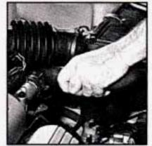
Start the engine and let it run until you can feel the upper radiator hose getting hot. Watch out for the engine fans.
