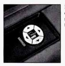
If your Buick has the optional power mirror, the mirror control is located on the driver's door.
