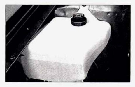
The coolant level should be at or above "FULL COLD." If it isn't, you may have a leak in the radiator hoses, heater hoses, radiator, water pump or somewhere else in the cooling system.
