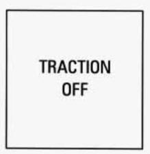
The "TRACTION OFF" warning light will come on when you turn the traction control system off. system off if you ever need to. (You should turn the system off if your vehicle ever gets stuck in sand, mud, ice or snow. See "Rocking Your Vehicle" in the Index.)
