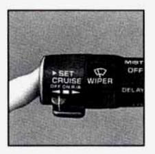
Push the button at the end of the lever, then release the button and the accelerator pedal. You'll now cruise at the higher speed. Here's the second way to go to a higher speed:
