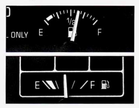
Your fuel gage shows about how much fuel is in your tank. It works only when the engine is on. When the indicator nears "E," you still have a little fuel left. You need to get more fuel right away. Here are four concerns some owners have had about the fuel gage. All these situations are normal and indicate nothing wrong with the fuel gage.
