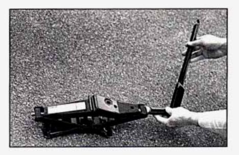
Using the wheel wrench, loosen all the wheel nuts. Don't remove them yet. Next, attach the wheel wrench to the bolt on the end of the jack. Raise the jack a little by rotating the wheel wrench clockwise (to the right).
