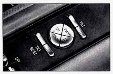
The power seat controls are located on the armrest. **Front Control (F):** Raise the front of the seat by pushing the left side of the switch Push the right side of the switch to lower the front of the seat.
