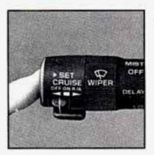
Push in the set button at the end of the lever and release it. (The "CRUISE" light on the instrument panel will come on.)
