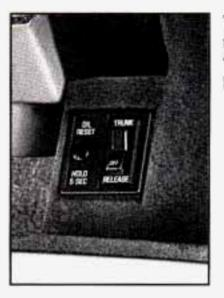
The trunk release switch in the glove box must be "ON" for the "TRUNK" button to work.
