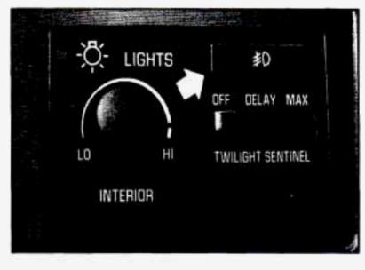
Use your fog lamps for better vision in foggy or misty conditions. When you press the upper fog lamp switch, a small indicator light will glow to tell you the fog lamps are on. Press the switch again to turn them off.
