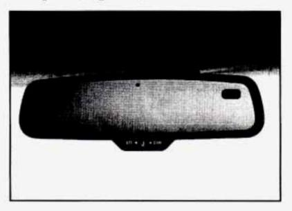
This mirror automatically changes to reduce glare when set in the M (Mirror) or C/M (Compass/Mirror) positions. One photocell on the back of the mirror senses when it is becoming dark outside. Another photocell is built into the mirror surface to sense headlamps behind you.
