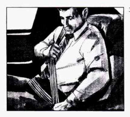
To make the lap part tight, pull down on the buckle end of the belt as you pull up on the shoulder part.
