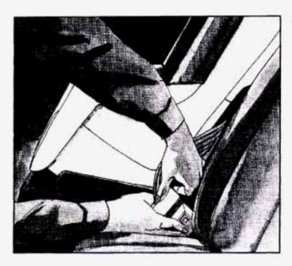
Buckle the belt. Make sure the release button is positioned so you would be able to unbuckle the safety belt quickly if you ever had to.
