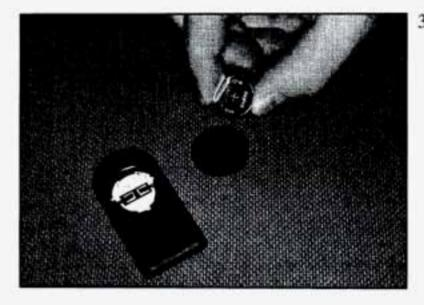
Make sure the battery is positioned with the "plus" (+) sign facing the cover.
