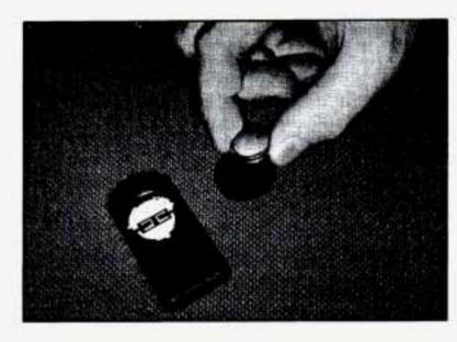
Remove the battery and replace with CR2025 or an equivalent. Using the wrong size battery can damage the transmitter.
