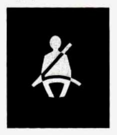
When the key is turned to RUN or START, a chime will come on for about eight seconds to remind people to fasten their safety belts. The safety belt light will also come on and stay on for about 75 seconds. If the driver's belt is already buckled, neither the chime nor the light will come on.
