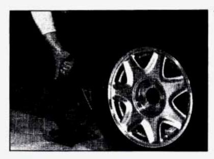
Raise the vehicle by rotating the wheel wrench clockwise.
