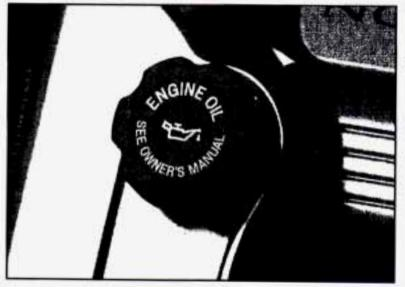
To remove, turn the oil fill cap counterclockwise.
