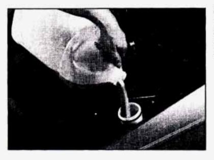
Open the cap labeled WASHER FLUID ONLY. Add washer fluid until the tank is full.
