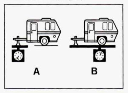
If you're using a "dead-weight" hitch, the trailer tongue (A) should weigh 10% of the total loaded trailer weight (B). If you have a "weight-distributing" hitch, the trailer tongue (A) should weigh 12% of the total loaded trailer weight (B).
