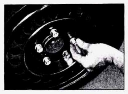
Replace the wheel nuts with the rounded end of the nuts toward the wheel. Tighten each nut by hand until the wheel is held against the hub.
