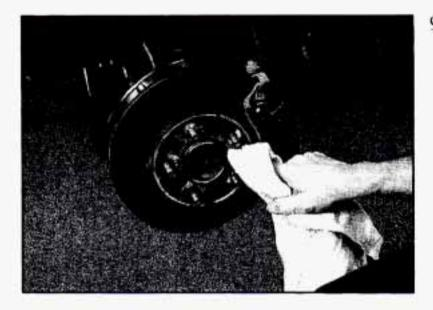
Remove any rust or dirt from the wheel bolts, mounting surfaces and spare wheel. Place the spare on the wheel mounting surface.
