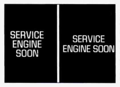
A computer monitors operation of your fuel, ignition and emission control systems. One of these lights should come on when the ignition is on, but the engine is not running, as a check to show you it is working. If one of these lights doesn't come on, have it fixed right away.
