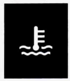
This light tells you that your engine has overheated. You should stop the car and turn the engine off as soon as possible. A warning chime should also sound if this light comes on.
