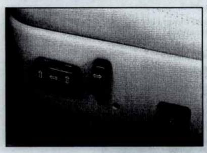
The power seat control switches are located on the outboard side of the front seat cushion.
