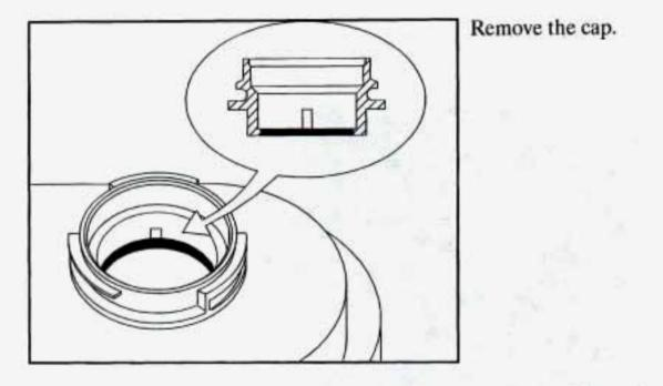
The fluid level must be to the maximum fill line at the base of the neck as shown.
