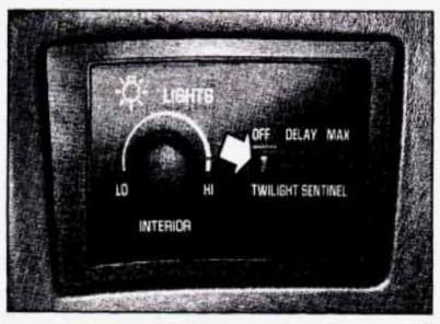
The control is next to the headlamp switch. It automatically switches your lamps on and off by sensing how dark it is outside. To operate the twilight sentinel, leave the lamp switch off and move the control to any position but OFF.
