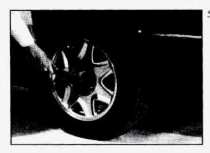
Using the wheel wrench loosen all the wheel nuts. Don't remove them yet.
