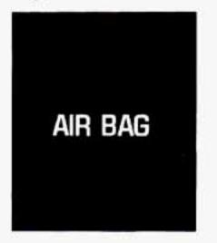
You will see this light flash for a few seconds when you turn your ignition to RUN or START. Then the light should go out. This means the system is ready.
