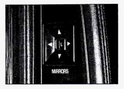
The control on the driver's door armrest operates both outside rearview mirrors. Move the center switch to the left to select the driver side mirror, or to the right to select the passenger side mirror. Then press the control pad in the direction of the desired mirror movement. Adjust each mirror so that you can just see the side of your vehicle.
