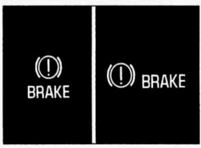
Your Cadillac's hydraulic brake system is divided into two parts. If one part isn't working, the other part can still work and stop you. For good braking, though, you need both parts working well.
