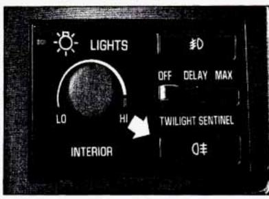
To operate the rear fog lamps, first turn on the front fog lamps, then press the lower switch. A small indicator light will glow to tell you they are on. Press the switch again to turn them off.
