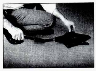
Attach the wheel wrench to the jack bolt and rotate it clockwise. That will raise the lift head a little.
