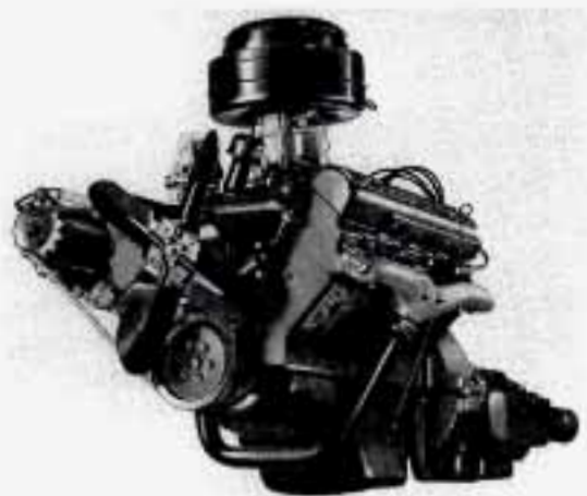
1949 Overhead Valve High Compression V8 Engine
