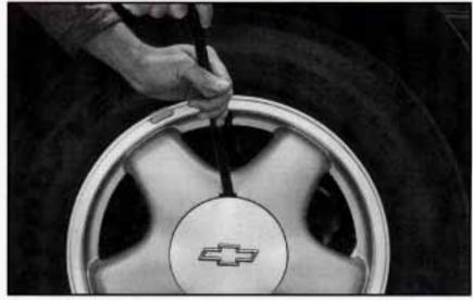
If there is a wheel cover, loosen the nut caps with the wheel wrench. They won't come off. Then, using the flat end of the wheel wrench, pry along the edge of the wheel cover until it comes off. Be careful; the edge may be sharp. Don't try to remove the cover with your bare hands.
