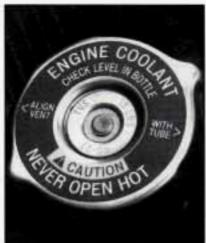
10. Then replace the pressure cap. At any time during this procedure if coolant begins to flow out of the filler neck, reinstall the pressure cap. Be sure the arrows on the pressure cap line up like this.
