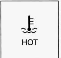
This light tells you that your engine coolant has overheated or your radiator cooling fan(s) are not working.
