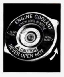
You can remove the radiator pressure cap when the cooling system, including the radiator pressure cap and upper radiator hose, is no longer hot. Turn the pressure cap slowly counterclockwise until it first stops. (Don't press down while turning the pressure cap.)
