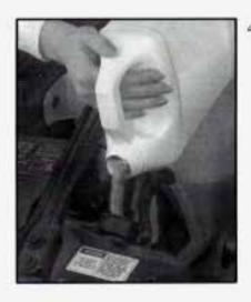
Fill the radiator with the proper DEX-COOL<sup>®</sup> coolant mixture, up to the base of the filler neck.
