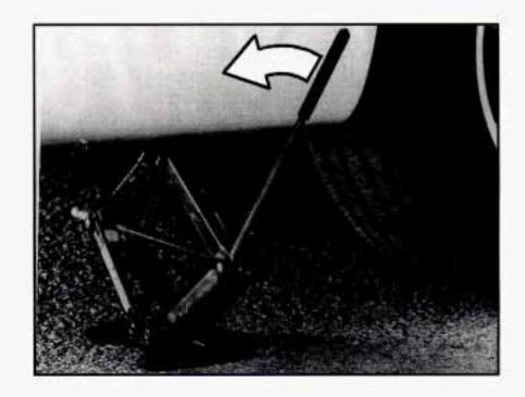
Lower the vehicle by turning the jack handle counterclockwise. Lower the jack completely.
