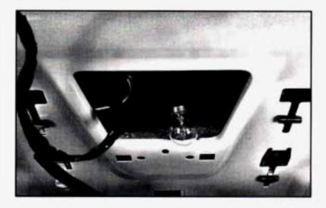
Open the trunk lid. Locate the stoplamp behind the rear seats, in front of the trunk hinges.
