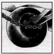
Attach a separate safety chain around the outboard end of both lateral arms.
