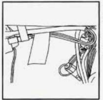
Your vehicle is equipped with auxiliary power leads. These leads can be used to power aftermarket electrical equipment added to your vehicle. They are located on the passenger's side of the vehicle, below the glove box and behind what is referred to as a "hush panel." For additional information on accessing these leads and electrical hookup, please refer to your service manual.
