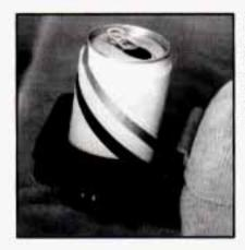
To use the storage area, fold down the armrest. Press the latch on the front edge and pull up. To use the cupholder, flip it forward.
