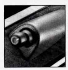
The power mirror control is on the driver's door. Turn the control to the left to adjust the left mirror or to the right to adjust the right mirror. Then move the control in the direction you want to move the mirror.
