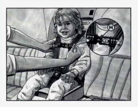
Now fasten the left and right halves of the shoulder harness clip together. The indicator window (H) on the clip will show green when the two halves are fastened together. The purpose of this clip is to help keep the harness positioned on the child's shoulders.
