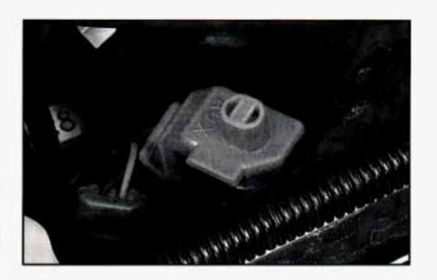
5. Find the positive (+) and negative (-) terminals on each battery. Your Chevrolet has a remote positive (+) jump starting terminal. The terminal is on the same side of the engine compartment as your battery. You should always use the remote positive (+) terminal instead of the positive (+) terminal on your battery. To uncover the remote positive (+) terminal, lift the red plastic cap.
