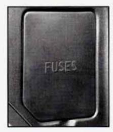
Some fuses are in a fuse block on the passenger side of the instrument panel. Pull off the cover labeled FUSES to expose the fuses.
