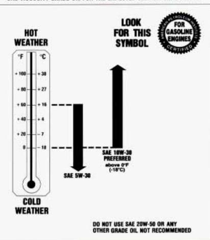
As shown in the chart, if you have the 3.4L DOHC engine, SAE 10W-30 is best for your vehicle. However, you can use SAE 5W-30 if it's going to be colder than 60°F (16°C) before your next oil change. When it's very cold, you should use SAE 5W-30. These numbers on an oil container show its viscosity, or thickness. Do not use other viscosity oils, such as SAE 20W-50.
