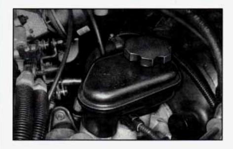
Your brake master cylinder reservoir is here. It is filled with DOT-3 brake fluid.
