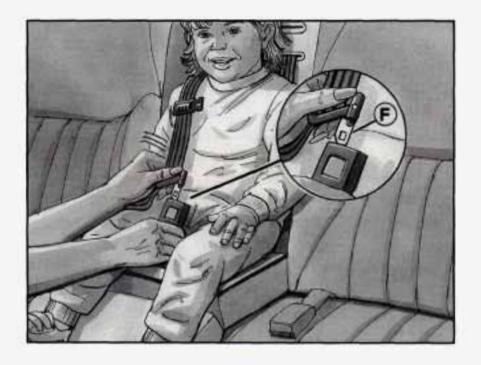
Select only one side of the harness. Pull the lap part of the harness out, and place the harness over the child's shoulder.
