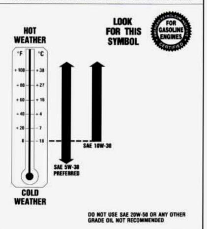
As shown in the chart, if you have the 3100 engine, SAE 5W-30 is best for your vehicle. However, you can use SAE 10W-30 if it's going to be 0°F (-18°C) or above. These numbers on an oil container show its viscosity, or thickness. Do not use other viscosity oils, such as SAE 20W-50.
