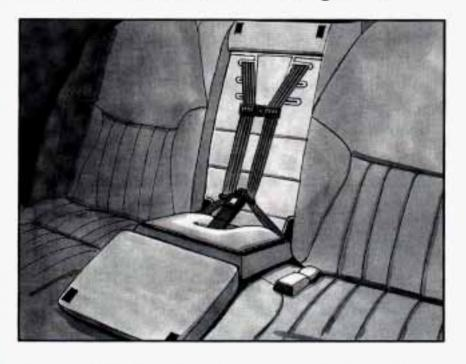
If your vehicle has this option, there's a built-in child restraint in the center rear seat position. This child restraint system conforms to all applicable Federal Motor Vehicle Safety Standards.
