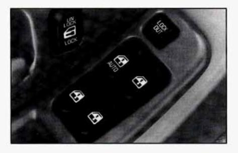
Switches on the driver's door armrest control each of the windows when the ignition is on. In addition, each of the passenger's doors has a switch for its own window. The driver's window switch has an auto-down feature. This switch is labeled AUTO. Tap the bottom of the switch, and the driver's window will open a small amount. If the bottom of the switch is pressed all the way down, the window will go all the way down.
