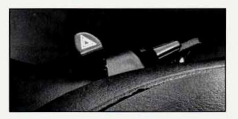
Press the switch (located near the ignition switch) to make your front and rear turn signal lamps flash on and off. Your hazard warning flashers work no matter what position your key is in, and even if the key isn't in.
