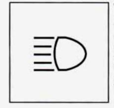
To change your headlamps from low beam to high beam, or high to low, pull the multifunction lever all the way toward you. Then release it. When the high beams are on, a light on the instrument panel also will be on.
