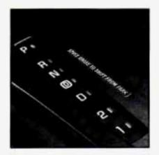
Your automatic transaxle may have a shift lever on the steering column or on the console between the seats.
