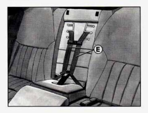
Now that the harness is adjusted to the correct height for your child, you're ready to use the child restraint's harness (E) to secure your child. Don't use the vehicle's safety belts.
