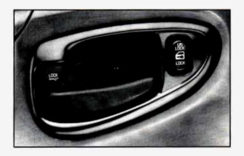
From the inside, push the lever to lock the door manually. To unlock, pull the lever.
