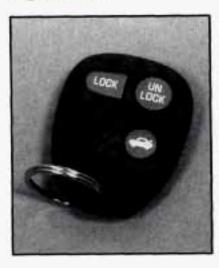
Press UNLOCK once to unlock the driver's door. Press UNLOCK again within five seconds to unlock all remaining doors; pressing UNLOCK will also cause the vehicle's interior lamps to come on for a period of time--(see "Sustained Interior Illumination" in the Index for more details).
