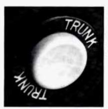
Press the button under the instrument panel on the driver's side. Your transaxle shift lever must be in PARK (P). Remember, your trunk can be opened at any time using this lock release, so be sure to lock your doors.
