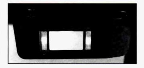
Open the cover to expose the vanity mirror. For the driver's mirror, slide the cover to the side. For the passenger's mirror, lift the cover. The lamps will come on when you open the cover on the passenger's visor.
