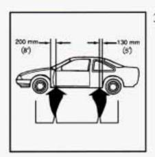
Position the jack under the vehicle and raise the iack lift head until it fits firmly into the notch in the vehicles frame nearest the flat tire.
