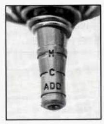
When the engine compartment is hot, the level should be at the H mark. When it's cold, the level should be at the C mark. If the fluid is at the ADD mark, you should add fluid.
