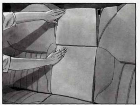
Then press the leg rest firmly into the seatback, and secure it by pressing the upper corners against the fastener strips on the seatback.
