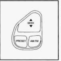
SEEK: Press the up arrow to tune to the next radio station and the down arrow to tune to the previous radio station.
