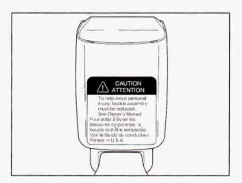
If you ever see a label on the driver's safety belt buckle that says to replace the buckle assembly, be sure to do so. Then the new buckle assembly will be there to help protect you in a collision.
