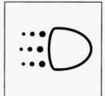
This light is on the instrument panel. It goes on whenever the DRL are on, the ignition is on, the headlamp switch is off and the parking brake is released.
