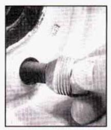
Put the nuts on by hand. Make sure the cone-shaped end is toward the wheel. Tighten each nut by hand until the wheel is held against the hub. If a nut can't be turned by hand, use the wheel wrench and see your dealer as soon as possible.
