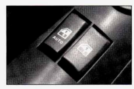
Press the side of the switch with the down arrow to lower the window.
