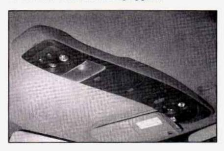
The overhead console includes reading lamps, a compartment for a garage door opener, a temperature and compass display and a storage compartment for sunglasses.
