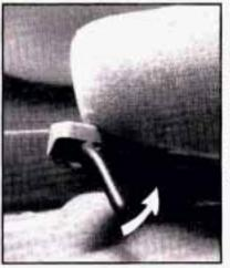
Move the lever under the front of the easy entry seat up to unlock it. Slide the seat to where you want it.
