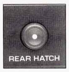
This button on the driver's side of the steering column allows you to release the rear glass from inside the vehicle.
