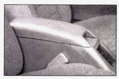
If your vehicle has this console compartment, squeeze the front lever while lifting the top to open it. You can store cassettes in the slots in the front of the compartment. If you have a compact disc player, you may store compact discs inside the console.
