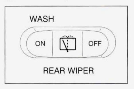
This switch is located on the instrument panel.
