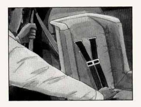
To tighten the belt, feed the shoulder belt back into the retractor while you push down on the child restraint.  Push and pull the child restraint in different directions to be sure it is secure. If you're using a bucket seat, adjust the seat forward until the lap portion of the safety belt holds the restraint firmly. But don't move it any more than needed to tighten the lap belt.
