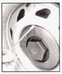
The optional hub cap removal tool is stowed with the jack.
