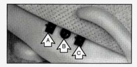
To make the front of the seat move up or down, use control A.
