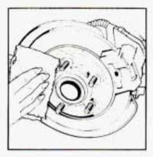
Remove any rust or dirt from the wheel holts mounting surfaces and spare wheel.
