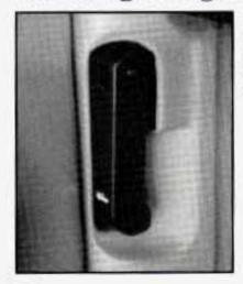
To open the hood, first pull the handle inside the vehicle on the lower driver's side of the instrument panel.
