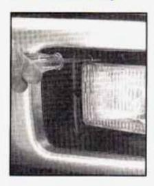
Remove the screws from the headlamp retainer.
