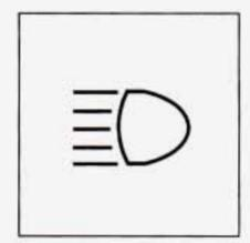
When the high beams are on, this indicator light on the instrument panel will also be on.
