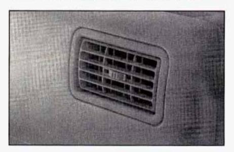
You will find air outlets in the center and on the sides of your instrument panel. You can move the outlets to direct the flow of air, or close the outlets altogether. When you close an outlet, it will increase the flow of air coming out of any outlets that are open.
