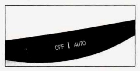
The right side of the switch located at the bottom of the mirror turns the electrochromic mirror on and off. To turn on the automatic dimming feature, press MIRROR. To turn off automatic dimming, press MIRROR again. The green indicator light will be illuminated when this feature is active.
