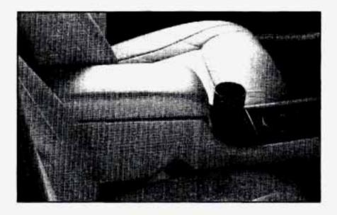
The console includes a storage compartment for CDs or tapes and an optional phone, an armrest and a cupholder. The cupholder can be opened by pressing on the surface panel located in front of the armrest. Close the lid to secure.
