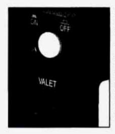
Pressing the VALET button located inside the glove box will disable the use of the power trunk, fuel door and garage door openers. Pressing this button again will make these features reusable. Locking the glove box with the door key will also help to secure your vehicle.
