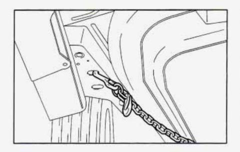
Attach R-hook chains to the R-hook slots in the frame rails just ahead of the rear wheels on both sides. These slots are to be used when loading and securing to car-carrier equipment.
