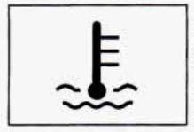
This light tells you that the engine has overheated. You should stop your vehicle and turn the engine off as soon as possible. A warning chime should also sound if this light comes on.
