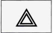
This light on the instrument panel will flash, indicating that the hazard warning flashers are on.
