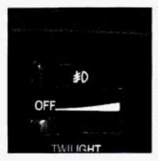
Use the fog lamps for better vision in foggy or misty conditions. When you press the fog lamp button, a small indicator light will tell you that the fog lamps and the parking lamps are on. Press the button again to turn them off.
