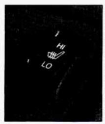
The control is located in the center console. Move the switch to LO or HI to turn on the heating elements in the seat. The LO setting warms the seatback and cushion until the seat approximates body temperature. The HI setting heats the seat to a slightly higher temperature.
