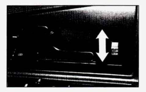
Press the power door lock switch to lock or unlock both doors at once.
