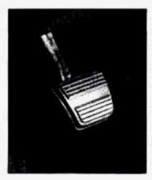
Hold the regular brake pedal down with your right foot and push down the parking brake pedal with your left foot to set the parking brake. If the ignition is on, the PARK BRAKE indicator light should come on. If it doesn't, you need to have your vehicle serviced.
