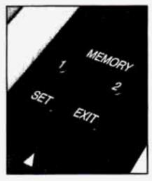
To begin programming, adjust the driver's seat (including lumbar adjustments) and both outside mirrors to a comfortable position and then press the SET button. Within five seconds, press button "1."
