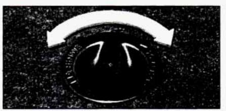
The equipment you'll need is in the trunk. Pull the carpeting from the floor of the trunk. Turn the retainer (center dial) on the compact spare cover to the left to remove it. Lift and remove the cover. (See "Compact Spare Tire" later in this section for more information about the compact spare.)
