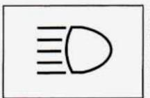
Pull the turn signal lever all the way toward you and then release it to change the headlamps from low beam to high or from high beam to low.
