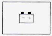
When you turn the key to RUN, this light will come on briefly to show that the generator and battery charging systems are working.
