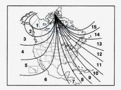
Press the COMPASS button on the bottom of the mirror until the new zone number appears in the display. After you stop pressing the button, the display will show a "C" in the direction display within a few seconds. (This is the automatic calibration mode -- you'll need to drive in a circle to calibrate the mirror. See "Compass Calibration" following.)
