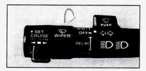
WIPER: Turn the band on the turn signal lever to control the wipers.
