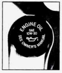
The oil fill cap is located behind the radiator on the passenger's side of the engine. Turn the cap to the left to remove it.
