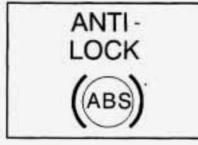
If there's a problem with the anti-lock brake system, this warning light will stay on. See "Anti-Lock Brake System Warning Light" in the Index.
