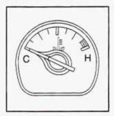
This gage shows the engine coolant temperature. If the gage pointer moves into the red area, the engine is too hot.
