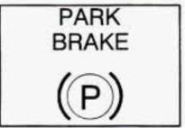
This light comes on when the parking brake is set, and it will stay on if the parking brake does not fully release. If you try to drive with the parking brake set, this light will remain on.
