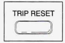
By pressing this button, you can tell how far you've traveled since you last set the trip odometer back to zero.
