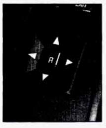
Your vehicle has an electric mirror control located on the driver's door armrest.
