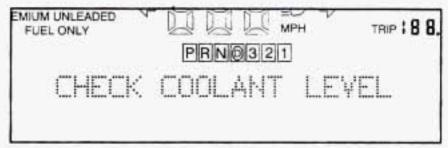
If the CHECK COOLANT LEVEL message comes on. it means you're low on engine coolant.
