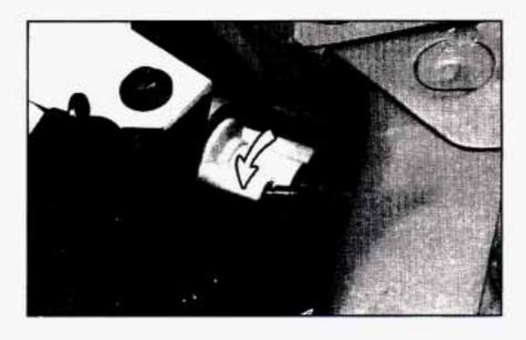
Turn the housing socket to the right to unlock the socket from the lamp housing.
