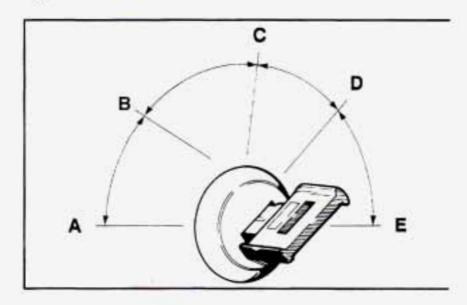
With the ignition key in the ignition, you can turn the switch to five different positions.
