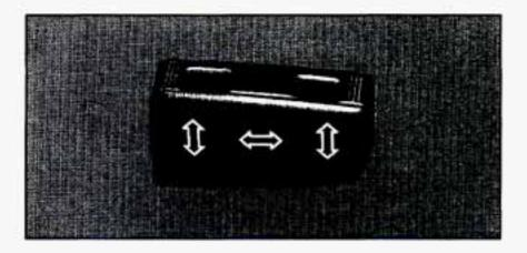
The power seat controls are located on the outboard side of the front seat cushion.
