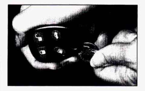
Use the round end of the door key or a coin to pry open the transmitter.
