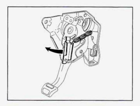
Be sure to turn off the ignition and put the vehicle in PARK (P) before manually releasing the brake.
