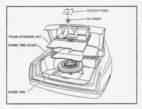
If equipped, the optional trunk storage system can be used to organize many different items inside the trunk.
