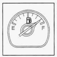
The fuel gage shows approximately how much fuel is in the tank. It works only when the ignition is in RUN.
