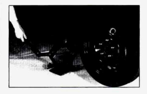
8. Lower the vehicle by rotating the wheel wrench to the left. Lower the jack completely.
