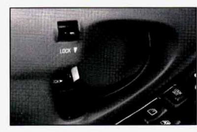
From the inside, to lock the door, move the locking lever forward.
