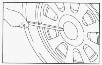
Some models are equipped with aluminum wheels. Remove the cover plate to find the wheel nuts. Carefully use the wedge end of the wheel wrench to pry it off.
