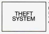
This light will come on briefly when you turn the ignition to ON. The light will stay on until the engine starts.
