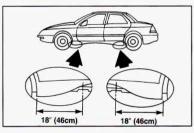
Position the jack and raise the jack head until it fits firmly into the notch in the vehicle's frame nearest the flat tire. Put the compact spare tire near you.
