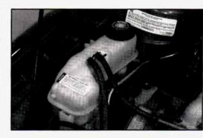
The coolant level should be at or above FULL COLD mark or slightly higher.
