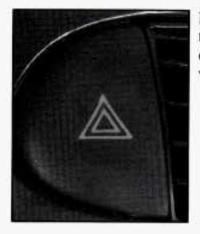
Press the switch once to turn your hazard flashers on. The switch will flash when activated.
