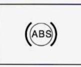
With the anti-lock brake system, this light will come on when you turn your ignition on or start your engine and it will stay on for three seconds. That's normal.
