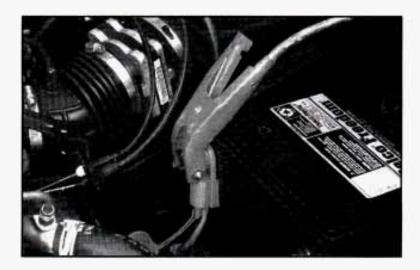
Connect the positive (+) cable to the positive (+) terminal of the vehicle with the dead battery. Use a remote positive (+) terminal if the vehicle has one.
