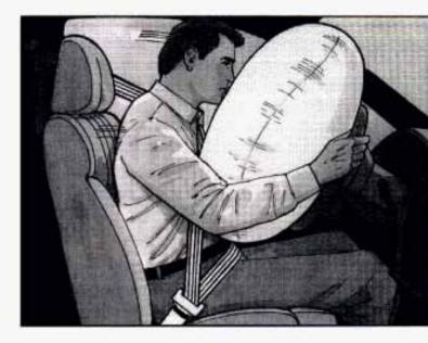
Where are the air bags? The driver's air bag is in the middle of the steering wheel.
