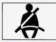
The safety belt light will also come on and stay on for about 20 seconds, then it will flash for about 55 seconds. If the driver's belt is already buckled, neither the chime nor the light will come on.
