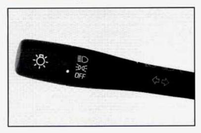
Rotate the turn signal lever end cap up one position to turn on:
