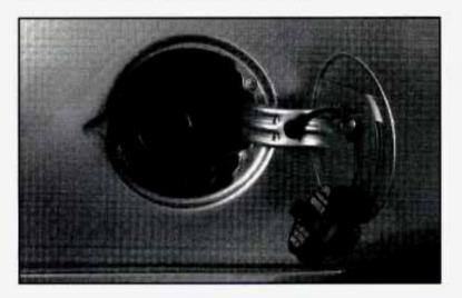
While refueling, hang the tethered cap inside the fuel door. To remove the cap, turn it slowly to the left (counterclockwise). The cap has a spring in it; if you let go of the cap too soon, it will spring back to the right.
