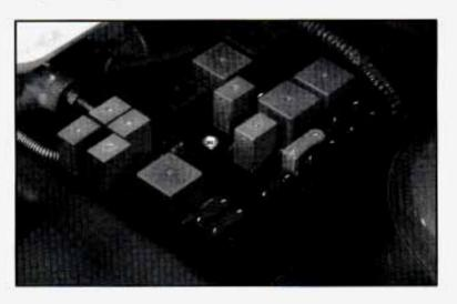
The engine compartment fuse block is located on the driver's side of the engine compartment, near the air cleaner.
