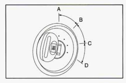
With the ignition key in the ignition switch, you can turn the switch to four positions.
