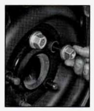
10. Replace the wheel nuts with the cone end of the nuts toward the wheel. Tighten each nut by hand or with the wheel wrench until the wheel is held against the hub.
