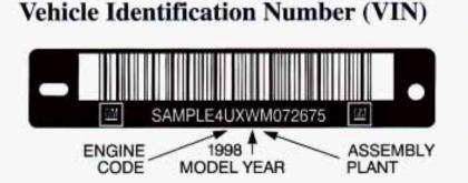
This is the legal identifier for your vehicle. It appears on a plate in the front corner of the instrument panel, on the driver's side. You can see it if you look through the windshield from outside your vehicle. The VIN also appears on the Vehicle Certification and Service Parts labels and the certificates of title and registration.
