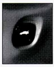
Press the remote trunk release button, located on the lower left side of the instrument panel, to release the trunk lid. Make sure the lockout feature is not activated. Also, the remote trunk release will only work when the gearshift lever is in PARK (P) or NEUTRAL (N).
