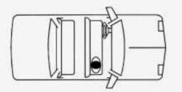
Your vehicle has a right front passenger air bag. Never put a rear-facing child restraint in this seat. Here's why:
