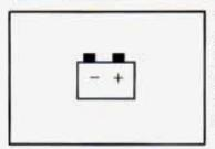
The charging system indicator light will come on when you turn on the ignition, but the engine is not running, as a check to show you it is working.
