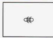
When the ignition is on, this light will stay on until all doors are closed and completely latched.
