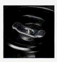
Turn the wing nut to the left and remove it. Then lift off the adapter and remove the spare tire.
