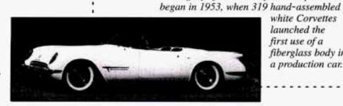
white Corvettes launched the first use of a fiberglass body in a production car.
