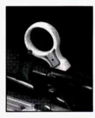
The engine oil dipstick on the 2.4L engine is located at the rear of the engine.
