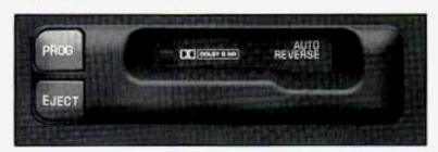
With this option, the remote single cassette player is mounted near the bottom of the instrument panel, above the ashtray and below the HVAC controls.
