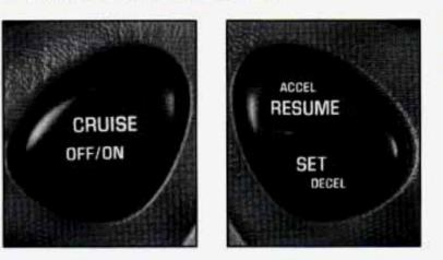
With cruise control, you can maintain a speed of about 25 mph (40 km/h) or more without keeping your foot on the accelerator. This can really help on long trips. Cruise control does not work at speeds below 25 mph (40 km/h).
