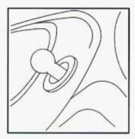
Adjust the driver's side outside mirror with the control lever on the driver's door.
