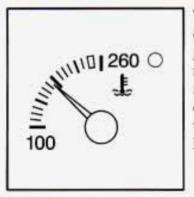
This gage shows the engine coolant temperature. If the gage pointer moves into the red area, the light comes on and you hear a chime, your engine is too hot! It means that your engine coolant has overheated.
