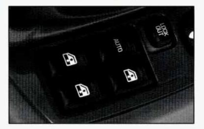
The power window switches are located on the armrest of the driver's door. In addition, each passenger door has a switch for its own window.
