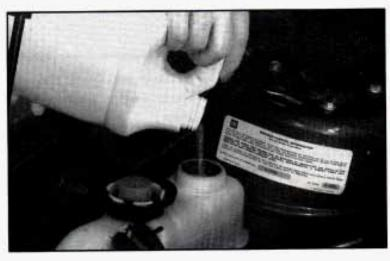
Then fill the coolant surge tank with the proper mixture, up to FULL COLD mark or slightly higher.
