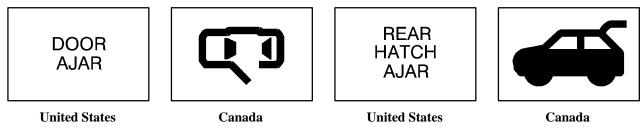
This message will come on when the ignition is turned to ON or START and the driver's or passenger's door is open. This message will come on when the ignition is turned to ON or START and the liftgate or tailgate is open.
