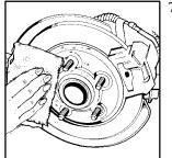
7. Remove any rust or dirt from the wheel bolts, mounting surfaces and spare wheel.
