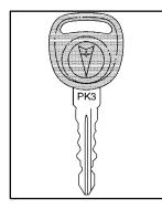
Your vehicle is equipped with the PASS-Key III (Personalized Automotive Security System) theft-deterrent system. PASS-Key III is a passive theft-deterrent system. This means you don't have to do anything different to arm or disarm the system. It works when you insert or remove the key from the ignition.
