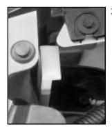
2. Push in on the headlamp and lift up the headlamp retaining clip partway, but do not remove.
