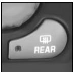
Press the REAR button to warm the defogger grid on the rear window. The engine must be running for the defogger grid to warm up.
