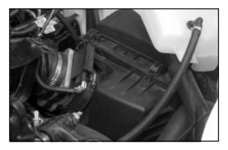
The engine air cleaner/filter is located at the front of the engine compartment on the driver's side of the vehicle, under the engine coolant reservoir.
