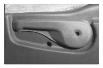
To adjust the seatback, pull up on the recliner lever located on the outboard sides of both the driver's and front passenger's seat.
