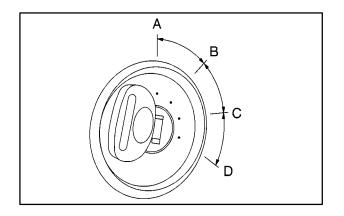
A (OFF): This is the only position from which you can remove the key. This position locks the steering wheel, ignition and transaxle.
