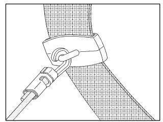
2. Attach the elastic cord to the comfort guide on the center passenger shoulder belt.
