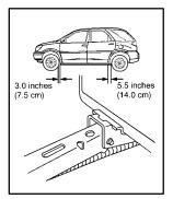
3. Near each wheel, there is a notch in the vehicle's body. Position the jack and raise the jack head until it fits firmly into the notch in the vehicle's frame nearest the flat tire.
