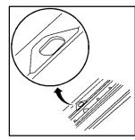
Use the four tie-down loops in each of the side rails to help secure large loads.
