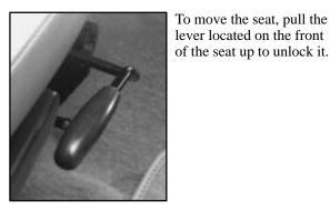
Slide the seat to where you want it and release the lever. To make sure the seat is locked into place, try to move the seat with your body.
