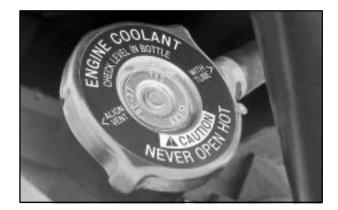
1. You can remove the radiator pressure cap when the cooling system, including the radiator pressure cap and upper radiator hose, is no longer hot. Turn the pressure cap slowly counterclockwise until it first stops. (Don't press down while turning the pressure cap.)
