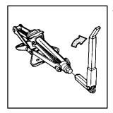
4. Attach the folding wrench to the jack, and turn the wrench clockwise to raise the jack head 3 inches (7.6 cm).
