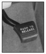
To set the parking brake, hold the regular brake pedal down with your right foot and push down on the parking brake pedal with your left foot.
