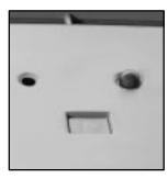
A light located on top of the instrument panel (near the center of the vehicle, next to the windshield) will flash slowly to let you know that the system has been armed. While armed, the doors will not unlock with the power door lock switch.
