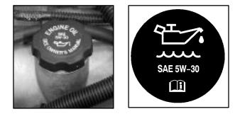
The engine oil fill cap is located just behind the engine oil dipstick. Your vehicle may have a cap with text and a graphic or just a graphic as shown above. See "Engine Compartment Overview" in the Index for more information on location.
