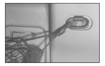
Attach both the upper and lower hooks to the loops on either side of the liftgate/tailgate opening (the label on the net should be in the upper left corner). Attach the middle hooks to the metal rings on the floor.
