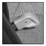
Lift up on the recliner lever located on the outboard side of the seatback.
