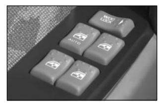
Switches on the driver's door armrest control each of the windows when the ignition is in ON, ACCESSORY, or when Retained Accessory Power (RAP) is active. See "Retained Accessory Power" in the Index. In addition, each passenger's door has a window switch.
