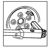
2. Loosen the wheel nuts -- but do not remove them -- using the folding wrench. (Turn the handle about 180 degrees, then flip the handle back to the starting position. This avoids taking the wrench off the lug nut for each turn.)
