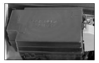
This fuse block is located in the engine compartment, to the rear of the windshield washer fluid reservoir.
