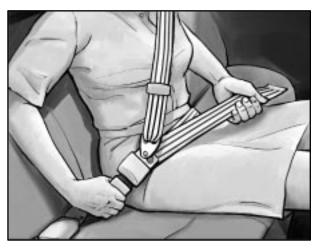
To make the lap belt longer, tilt the latch plate and pull it along the belt. To make the belt shorter, pull its free end as shown until the belt is snug.
