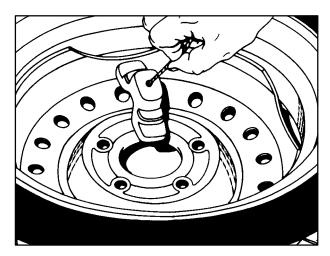
4. To remove the spare tire from the cable, tilt the retainer and slip it through the wheel opening.
