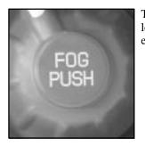
The fog lamp button is located in the center of the exterior lamps control.
