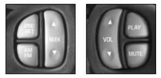
**PRESET:** Press this button to play a station you have programmed on the radio preset pushbuttons. The radio will go to a preset station, play for a few seconds, then go to the next station. Press this button again to stop scanning the preset stations. If a cassette tape is playing, press this button to play the other side of the tape.
