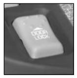
The power door lock switches are located on both the driver's and the front passenger's door armrests.
