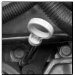
The engine oil dipstick is located at the front of the engine compartment, near the center. The dipstick handle has a bright, yellow loop design for easy identification.
