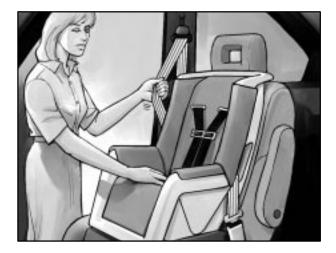
5. To tighten the belt, pull up on the shoulder belt while you push down on the child restraint. You may find it helpful to use your knee to push down on the child restraint as you tighten the belt. 6. Push and pull the child restraint in different directions to be sure it is secure.
