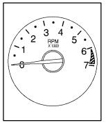
The tachometer displays the engine speed in revolutions per minute (rpm).
