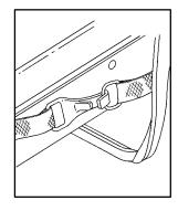
3. Disconnect the tethered ring from the hook and place the tethered ring on the outer edge of the tailgate on each side of the vehicle.
