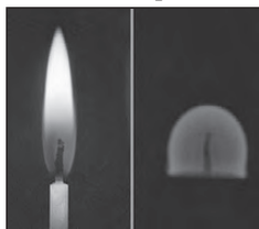
On Earth, flames form a teardrop shape (left). In microgravity, flames grow into a rounder shape.
