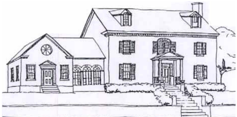
A side addition should be compatible with the design of the original building
