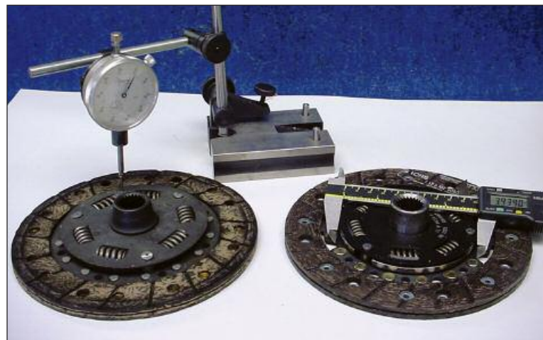
Clutch discs with a dial indicator on the hub of the aftermarket disc and a digital caliper measuring the Sachs hub diameter.
