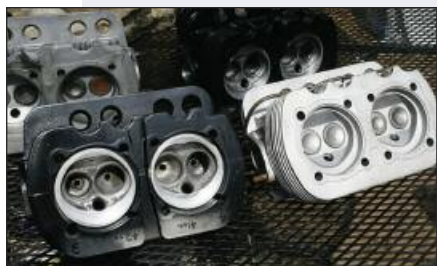
The 36 hp case is carefully drilled to allow oil to return to the sump with the least interference. Above: The heads of the larger valves are smooth and thin, chamber unshrouded, the ports are carefully modified for optimum flow. Each of these components is exhaustively tested on Tom's flow bench. The current heads, based on the original Okrasa style, took a year to develop and are known as the "Bruckrasa" heads. His approach has always been to out-think rather than out-spend competitors.
