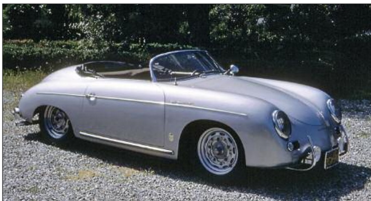
In 1966 Dana molded off the trunk handle, sprayed the car silver himself (the car's fifth paint job), added nerf bars, 15" wheels and driving lights.
