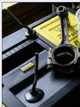
A Suzuki turbo engine is tough, but it still needs bearing oil. Inadvertently directing most oil to the turbo led to a rod failure, but Tom was amazed that no valves broke. Left: Specially modified Porsche 912 crank and cylinders to be used in the 1200 VW case. Below: Just part of his turbo stash.
