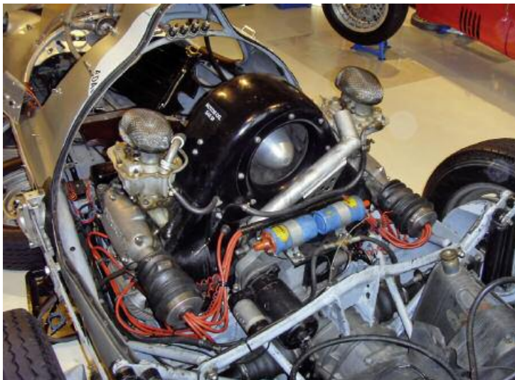
Right: In this photo by the author, you get a peek under the skin shows how compact the packaging is. It isn't all pretty, but it is effective. At the left, just inboard of the trailing arm you can see one tine of the "pickle fork" that was split and moved out-board.
