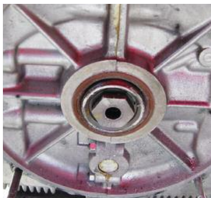
Above: The gland nut still holds the flywheel hub to the engine. Note the slight web of metal that held the flywheel.
