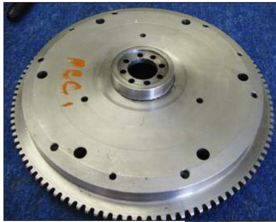
Left: The back of my improperly lightened flywheel. Note the excess material removed from the entire back with more removed from the inner hub area.
