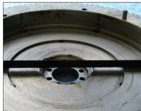
Below: The incorrectly machined flywheel. Note the lack of metal and contour under the straight edge. Bottom: Stock flywheel. Note contour of the hub area under the straight edge.
