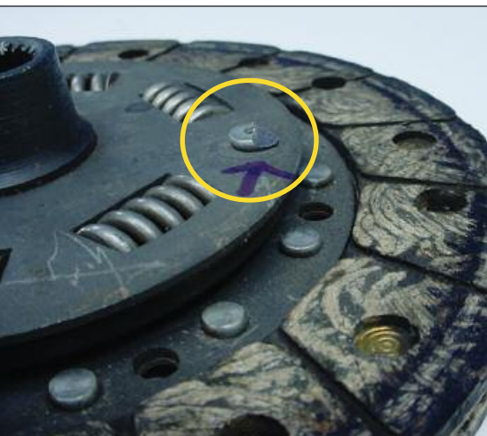
A close up of the aftermarket clutch disk. The arrow points to where the rivet had contacted the pressure plate.
