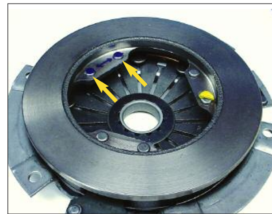
The arrow points to the pressure plate rivets. At the top, the arrow points to a rivet that had contact with the pressure plate. The clay (at about 3 o'clock) is peeled up. This was measured for clearance.
