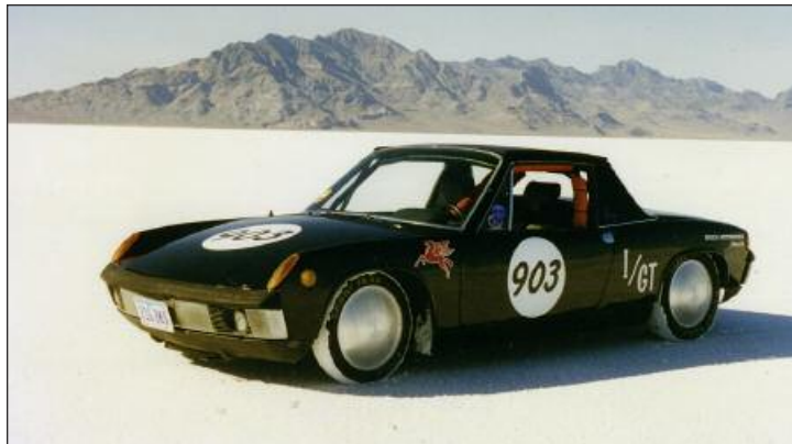
With the Schlaubaugh brothers, Tom built a 3-cylinder 1-liter 914 that still holds a class record. With a low-compression 2-liter 911 engine the car also captured that class with S pistons and 906 cams.
