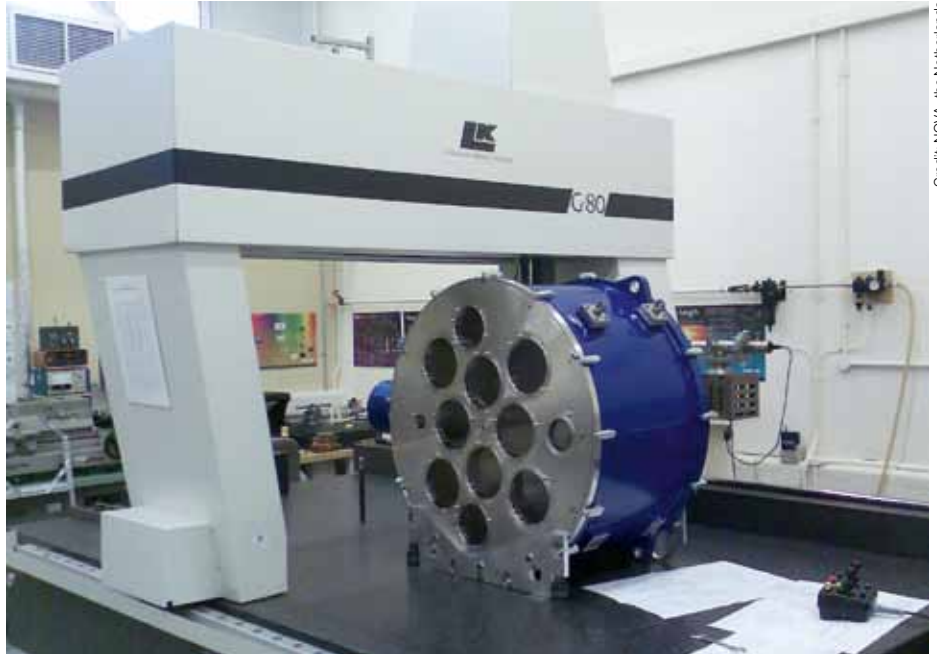
First ALMA front end assembly ready for acceptance testing at the European Front End Integration Centre (RAL, UK).
