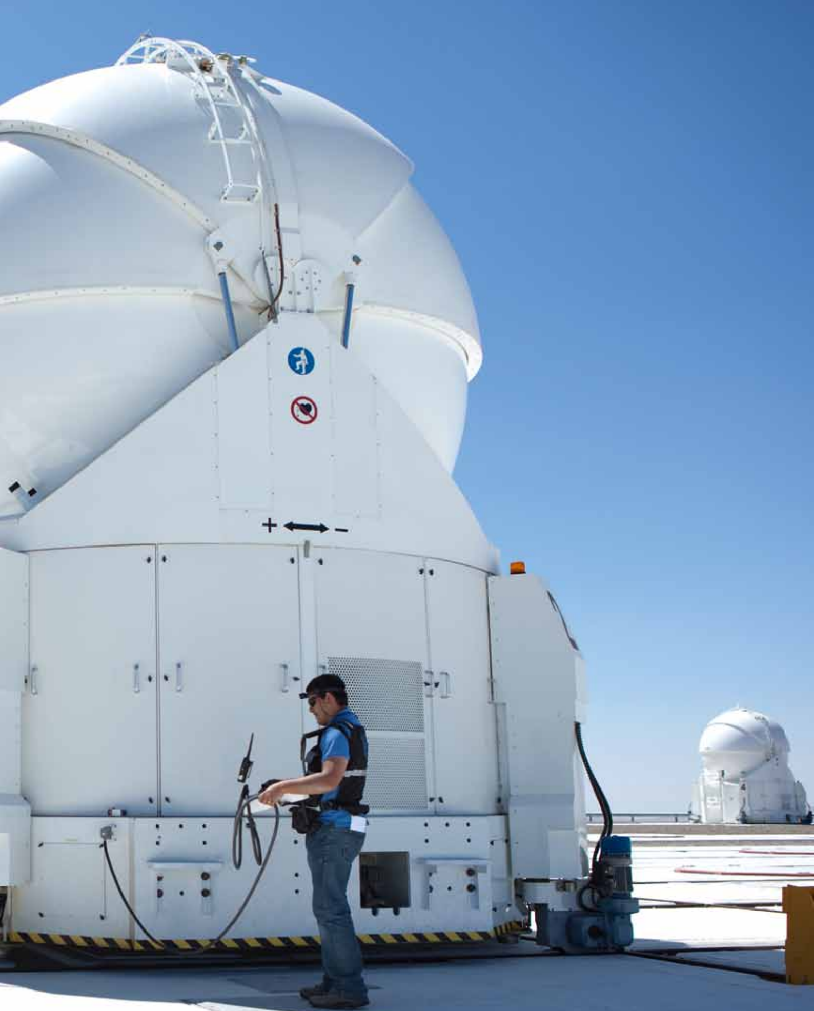
Auxiliary Telescope 2 arriving at its new observational position. This configuration with the other ATs is one of the most extreme for the interferometer.
