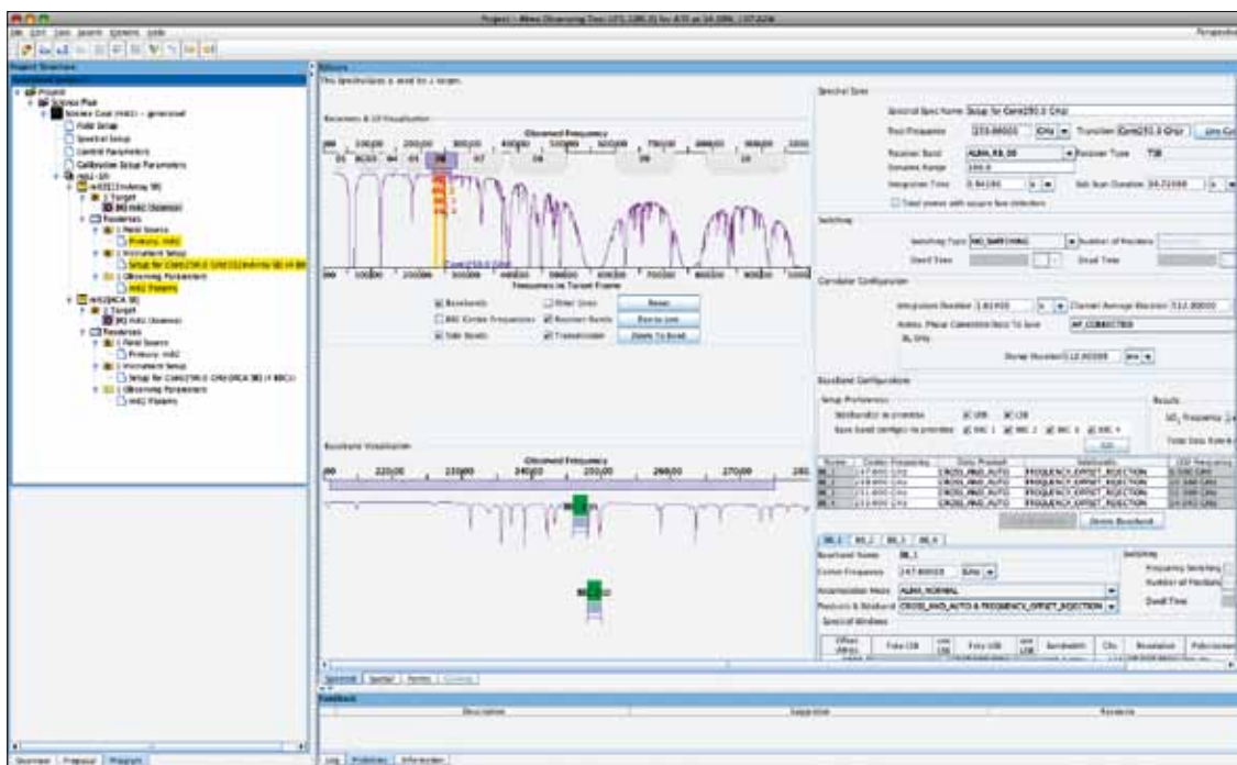
The ALMA Observing Tool (OT) is the main interface between users and the Joint ALMA Observatory (JAO) at the proposal and scheduling stage of a project. All proposals will be created and submitted to the JAO using the OT, which will also produce the observing scripts required to run the observations. The figure shows a typical view of the OT in its scheduling mode. A spectral visualisation of the receiver setup, including the atmospheric transmission curve (purple line), dominates the view. The tree on the left shows the structure of a typical project, which also includes observations with the ALMA Compact Array.
