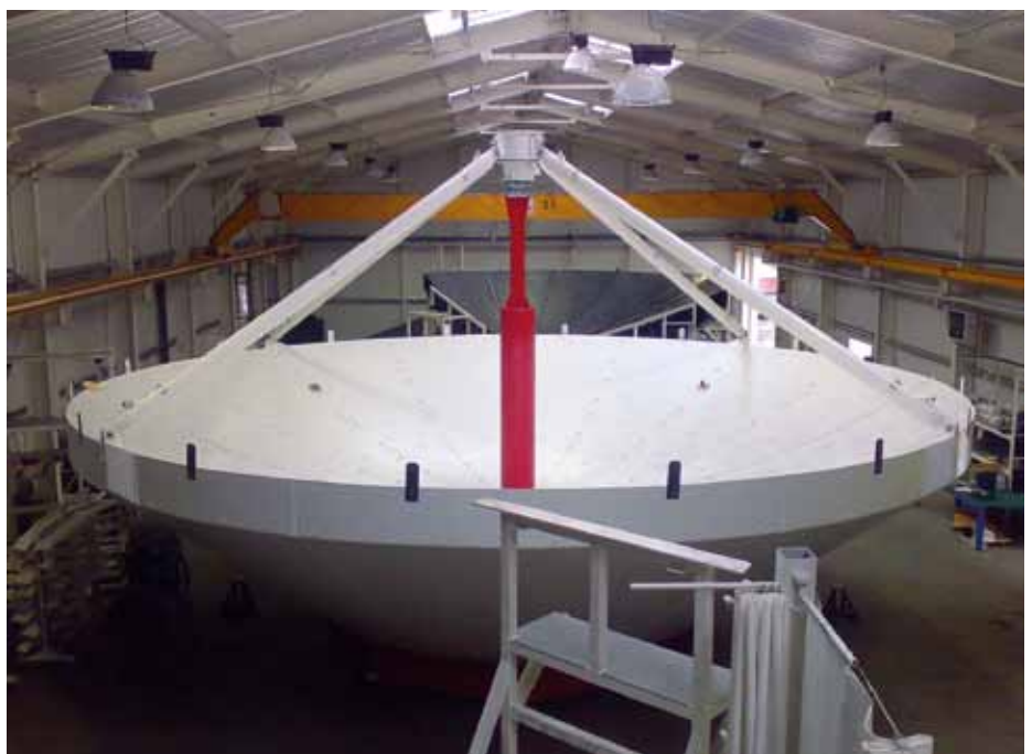
Antenna BUS at the manufacturer's premises.
