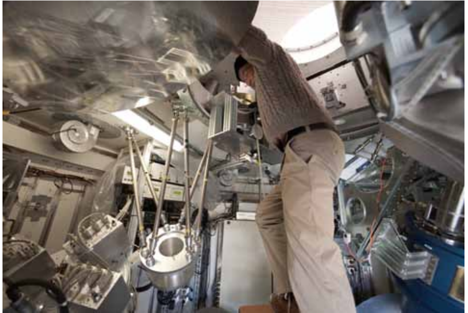
The SABOCA instrument being filled with helium.
