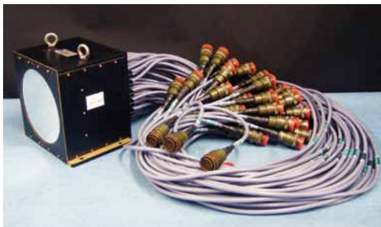
The 1377-actuator deformable mirror for the SPHERE instrument after delivery to ESO by the manufacturer CILAS.
