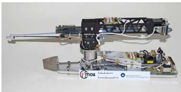
One of the 24 cryogenic R-theta robotic pickoff arms used by KMOS to select its targets.
