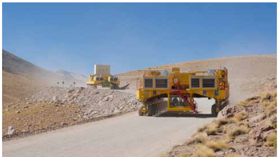
The two ALMA antenna transporters during tests between the OSF and the AOS. One is loaded with a "dummy antenna".
