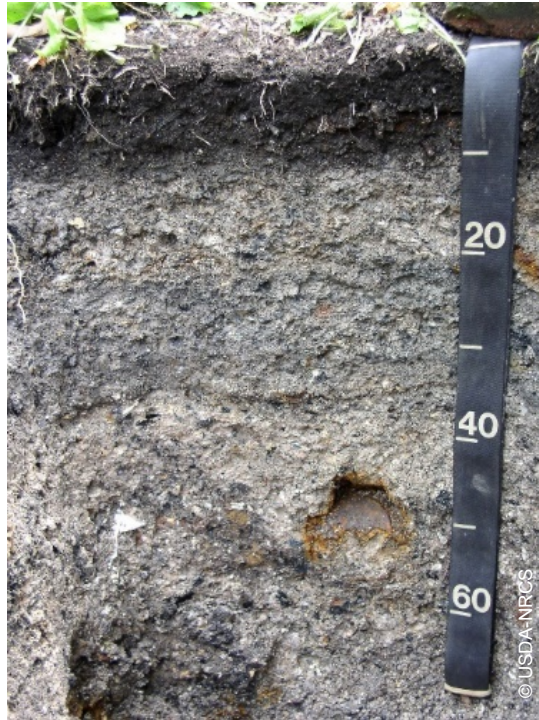
Photo 17. Soil profile, Combustic human-altered and human-transported (HAHT) material class. Mosholu soil series, Van Cortlandt Park, Bronx, NY, United States of America, containing 508.93 t SOC/ha
