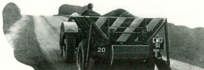
Ferguson Tractor used by West Riding of Yorkshire County Council towing a Gritter.
