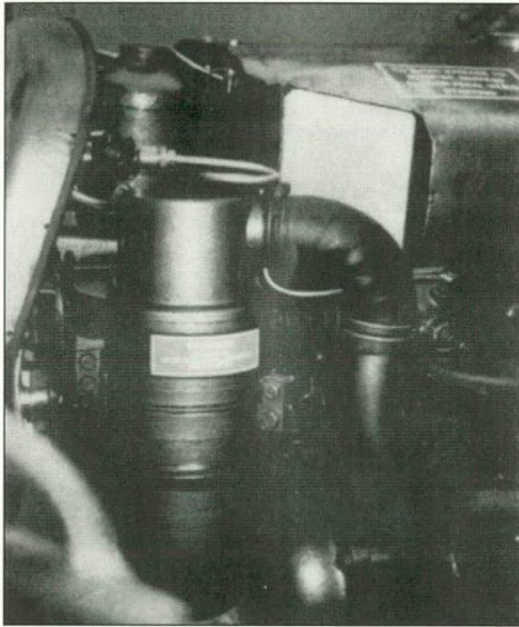
The new Ferguson Club transfers showing their correct positions on the air cleaner and fuel tank. Note that this tank is the later diesel type with full cutaway corner.
