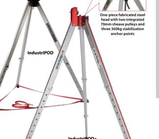
IndustriPOD+ Shown with (L) Fall Arrest Block Adaptor and winch and (R) Winch with Adaptor Bracket (not available USA)
