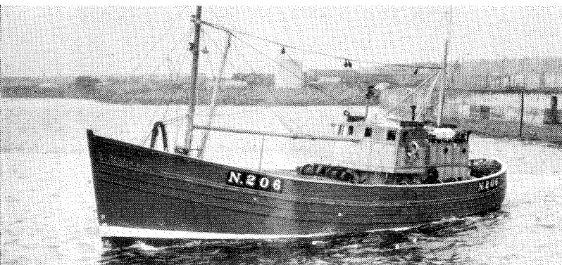
75 ft. trawler 'Castle Bay' built by J. G. Forbes of Sandhaven powered by a Caterpillar D343 engine supplied by Caledonia Motor Eqt. Ltd. This uses a MORSE MK Control.
