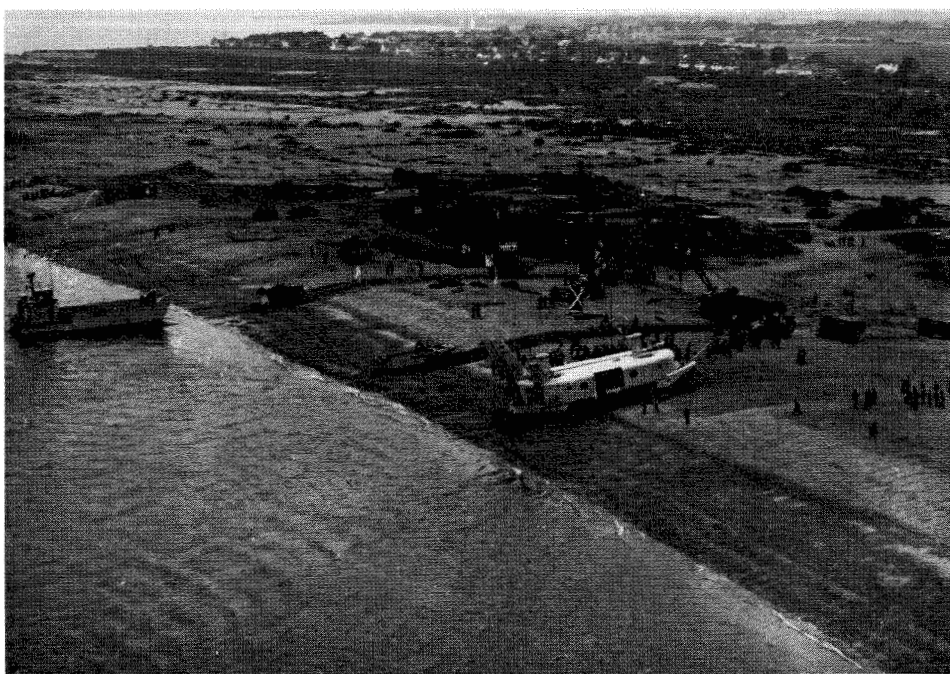
The 37-ton SR.N3 ashore at an Army training area in the British Inter-Service Hovercraft Trials Unit for military evaluation. The hovercraft's advantage over conventional landing craft is strikingly illustrated by this picture
