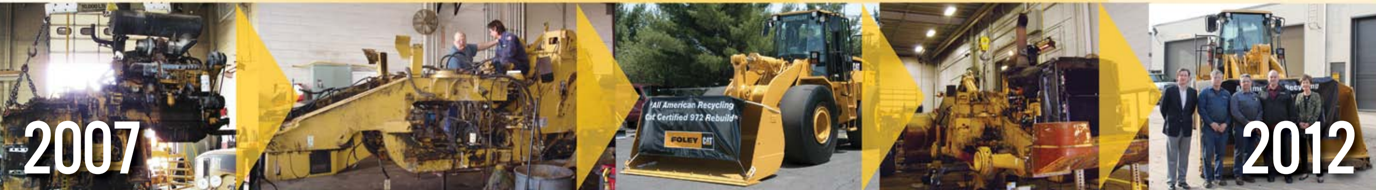
A Cat Certified Rebuild meant major dismantling of a used 972G loader in 2007.
