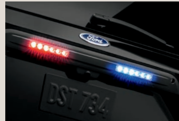
Rear auxiliary liftgate lights. Features backlit flashing, linear high-intensity LED lights (driver side red; passenger side blue) mounted just above the license plate.
