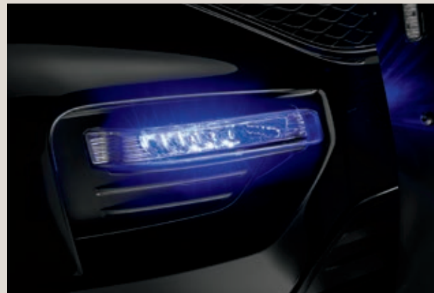
Front warning auxiliary lamps. Features integrated, custom-designed LED assemblies.
