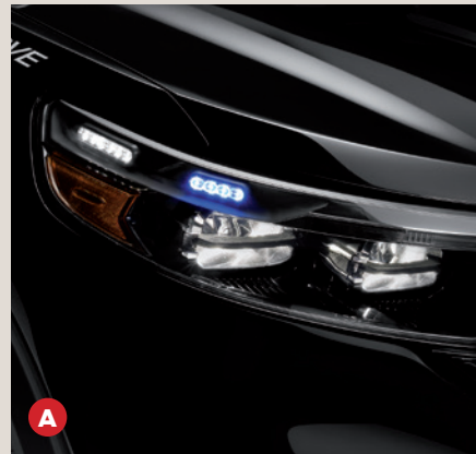
Front Headlamp Lighting Solution. Includes base headlamps with high-beam wig-wag function and (2) LED side warning lights (driver side red/white; passenger side blue/white).
