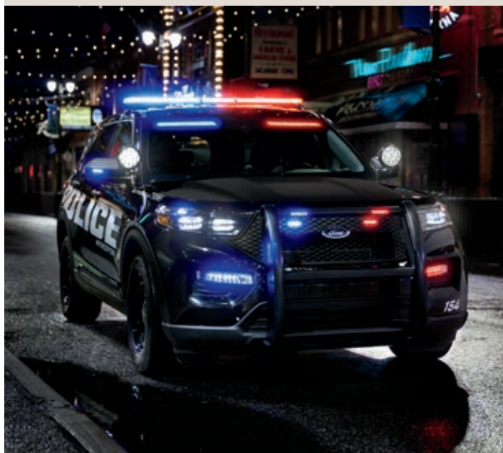
Front Headlamp Lighting Solution (66A). Includes base headlamps with LED high- and low-beam wig-wag function and LED side warning lights (driver side red/white; passenger side blue/white).
