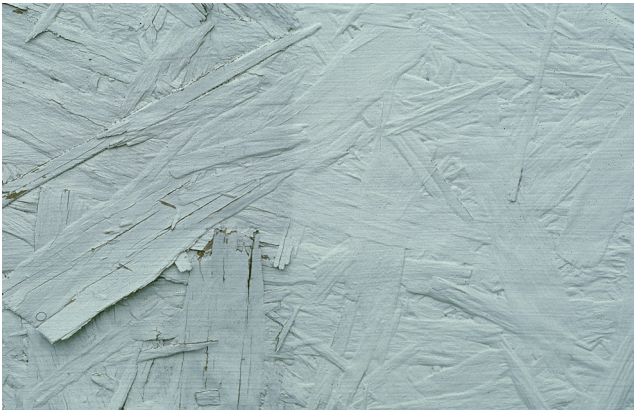
Figure 16–9. Absorption of water causes differential dimensional change of surface flakes and strands to give an uneven surface (telegraphing).
