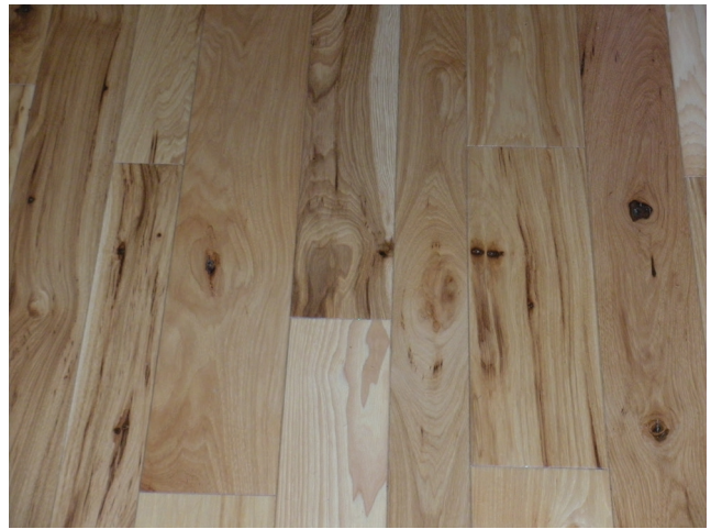
Figure 16–32. Number 2 grade of hickory with a transparent finish to accentuate the beauty of the various colors, knots, and grain pattern of this species.
