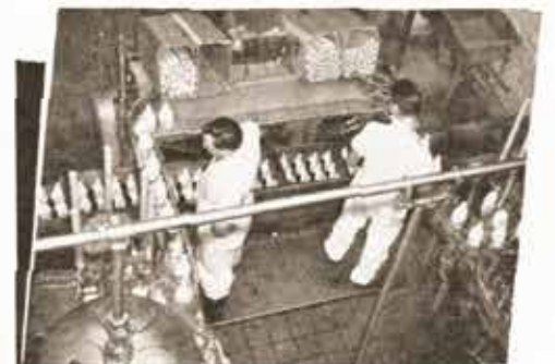
Movement of milk within the plant matches the efficient Truck-Trailer delivery. Bottles and store cartons are filled automatically on a production line at the rate of 300 quarts per minute—ready for the milkman's wagon.
