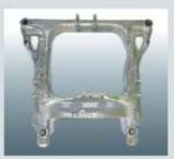
Aluminum front Subframe (Continuous weld by FSW\*)
