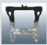
Steel and aluminum front Subframe (Welded two dissimilar metals by FSW\*)
