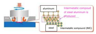
Joined by the intermetallic compound produced between the steel and aluminum
