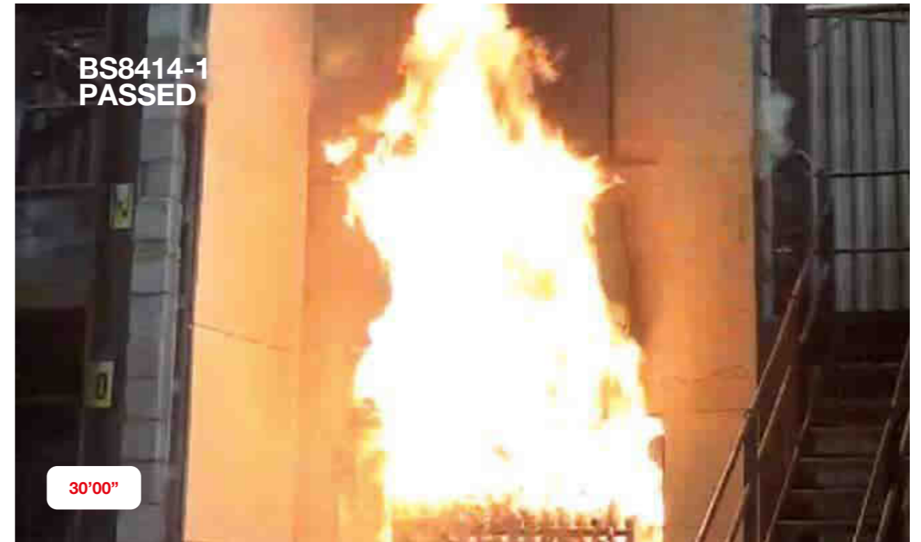
Reaction to fire of GammaStone AIR wall assembly after 30'00" of direct flame exposure
