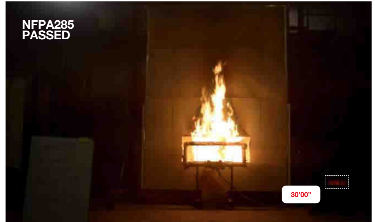
Reaction to fire of GammaStone AIR wall assembly after 30'00" of direct flame exposure
