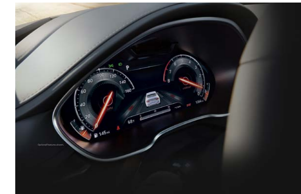
12.3" 3D DIGITAL INSTRUMENT CLUSTER
